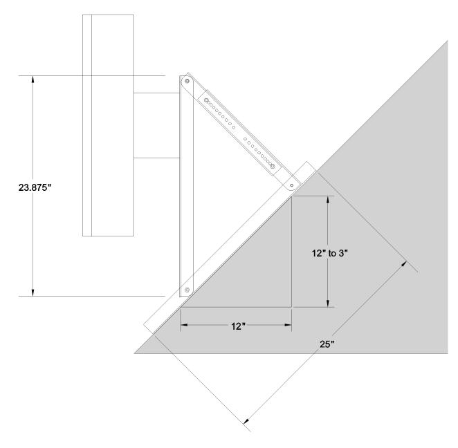
\*\*The above drawing is displaying a 24" bracket at a 12/3 roof pitch.
