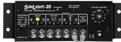
One 20 amp Lighting Controller will run up to 240 watts of sign load. These controllers can be ran in parallel if your sign is too large for one unit.
