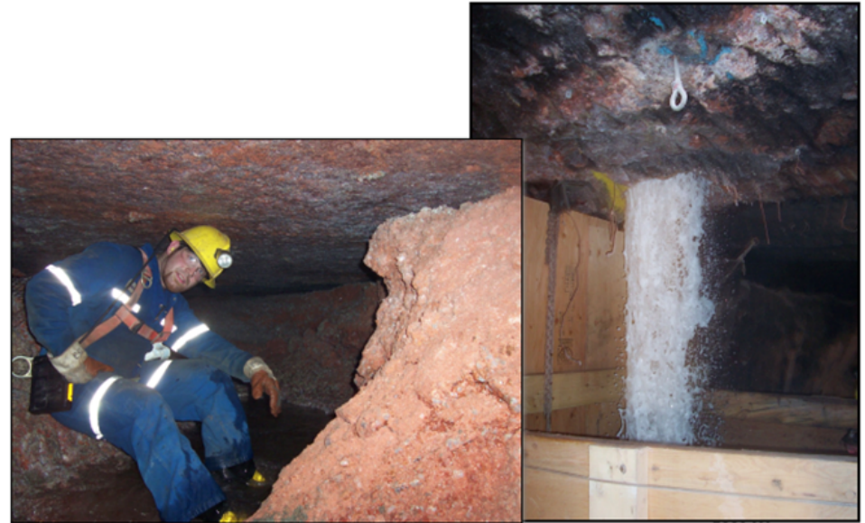
Fig. Inflow problems in a mine
