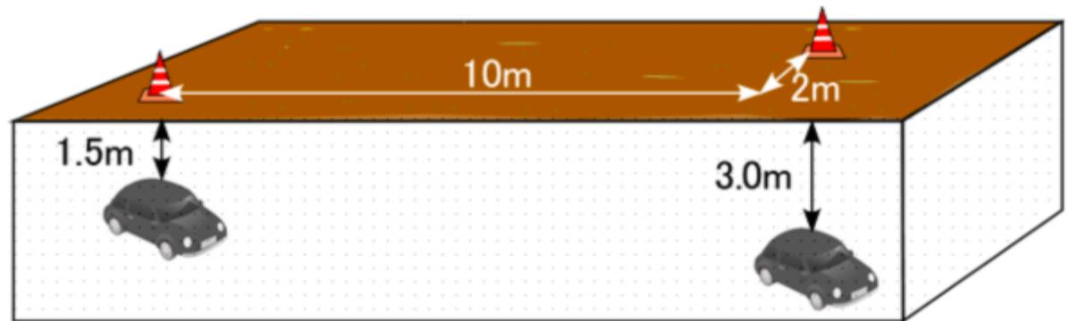
Fig. 4 Arrangement of the burial vehicle experiment site of the construction laboratory site
