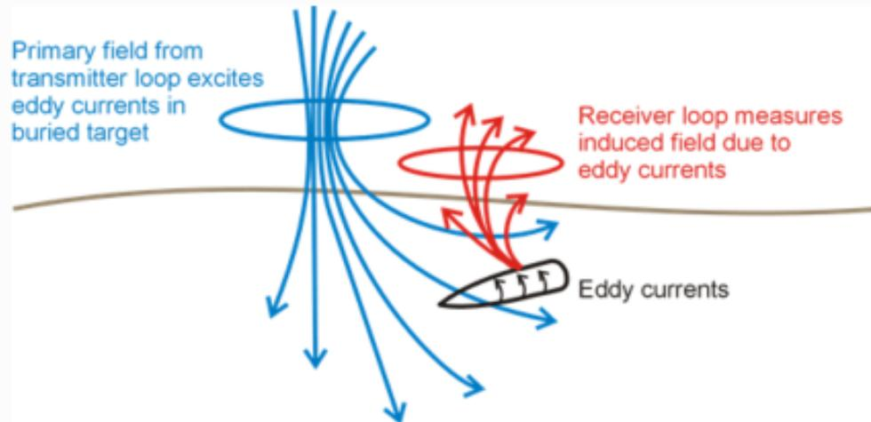
Fig. 260 Electromagnetic induction (EMI) survey for UXO location.
