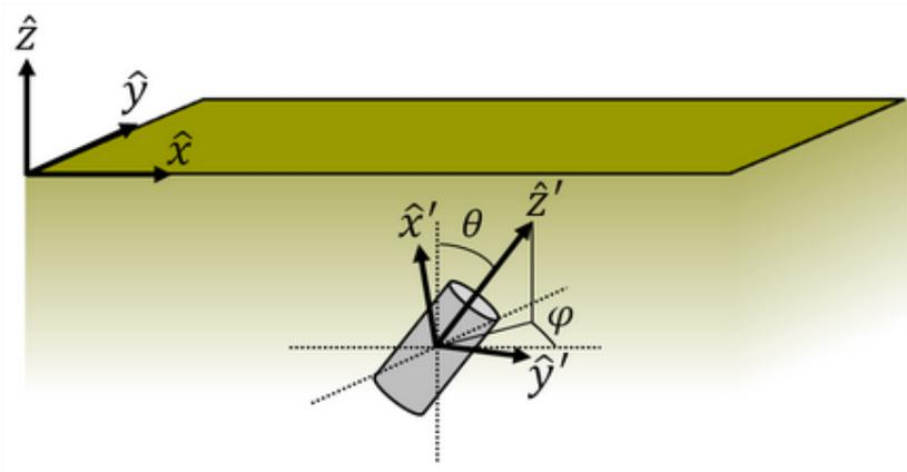
Primary (L1) and secondary (L2,L3) polarizations for UXO
