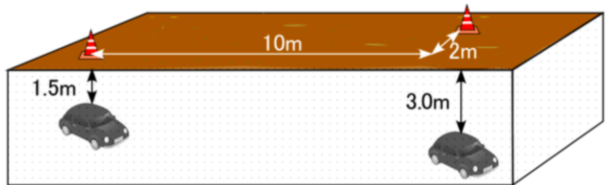
Fig. 4 Arrangement of the burial vehicle experiment site of the construction laboratory site Two buried mini vehicles are buried in the ground of 1.5 m depth and 3.0 m depth, respectively.
