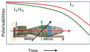
To carry out inversion for polarization tensor need data:
