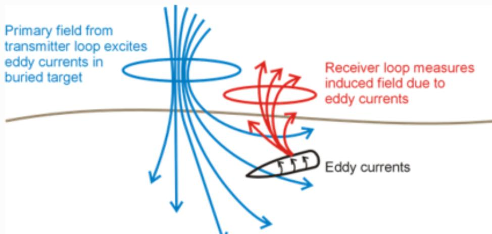
Fig. 260 Electromagnetic induction (EMI) survey for UXO location.
