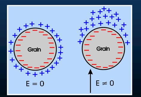
Schematic for polarization of electrical double layer of interconnected pore surface around a single mineral grain
