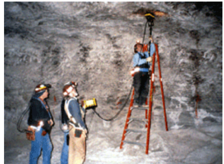
Fig. GPR survey along ceiling of a mine shaft. Courtesy of: https://www.sensoft.ca/
