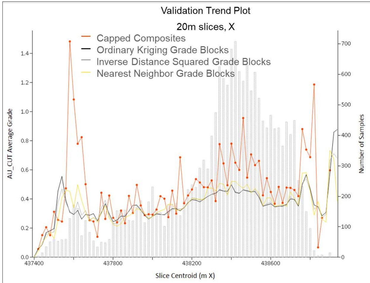
Figure 14-18: Block model validation swath plot along strike (X-direction)
