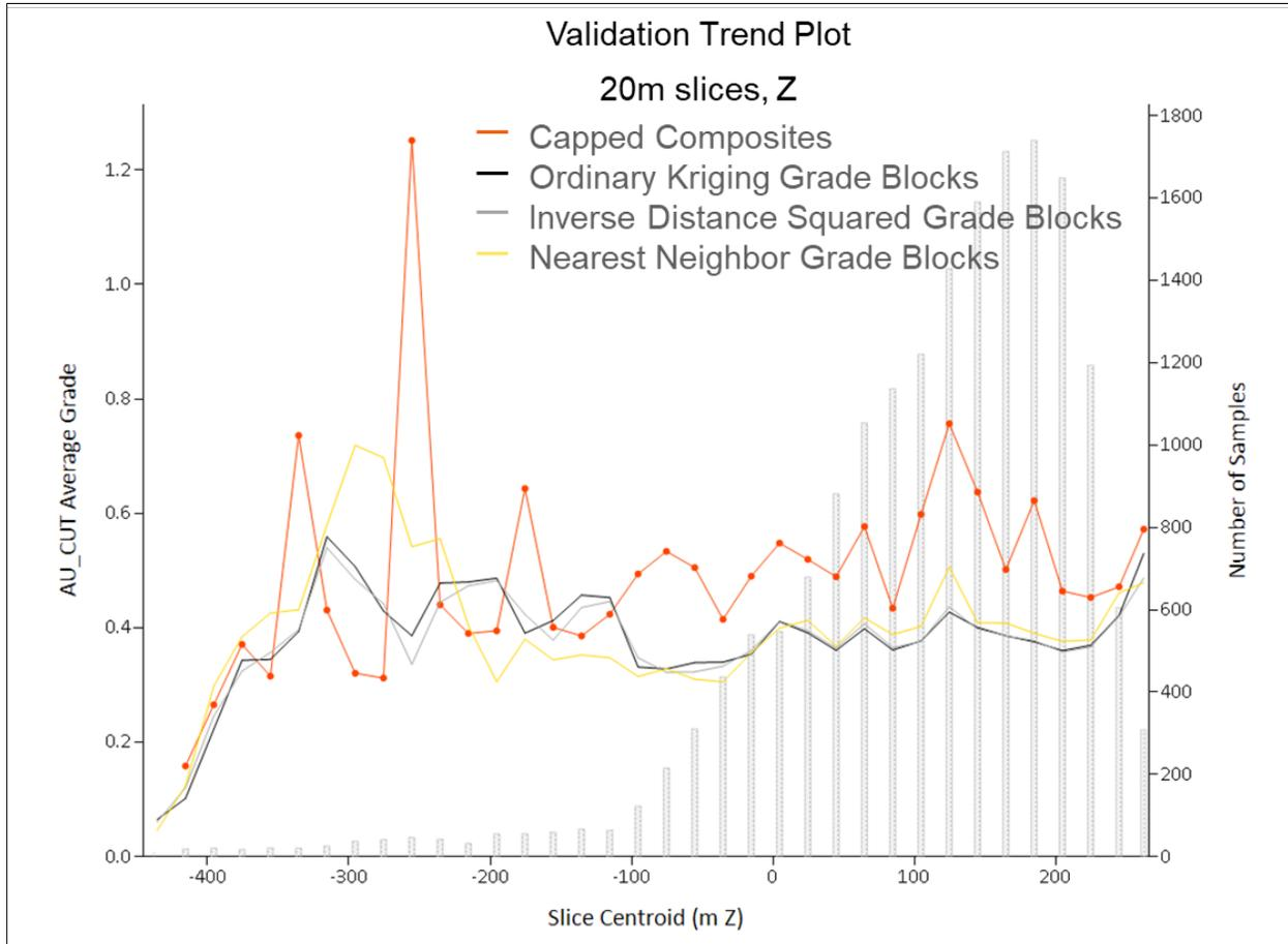
Figure 14-20: Block model validation swath plots along elevation (Z-direction)
