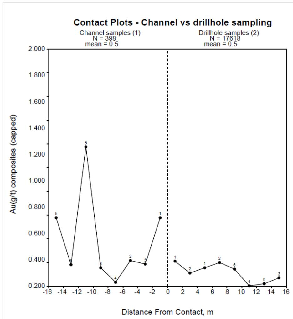
Figure 14-13: Contact analysis on the capped composites between the channel and the drillholes data (The number of pairs is low; this graph should be updated when more data is available.)
