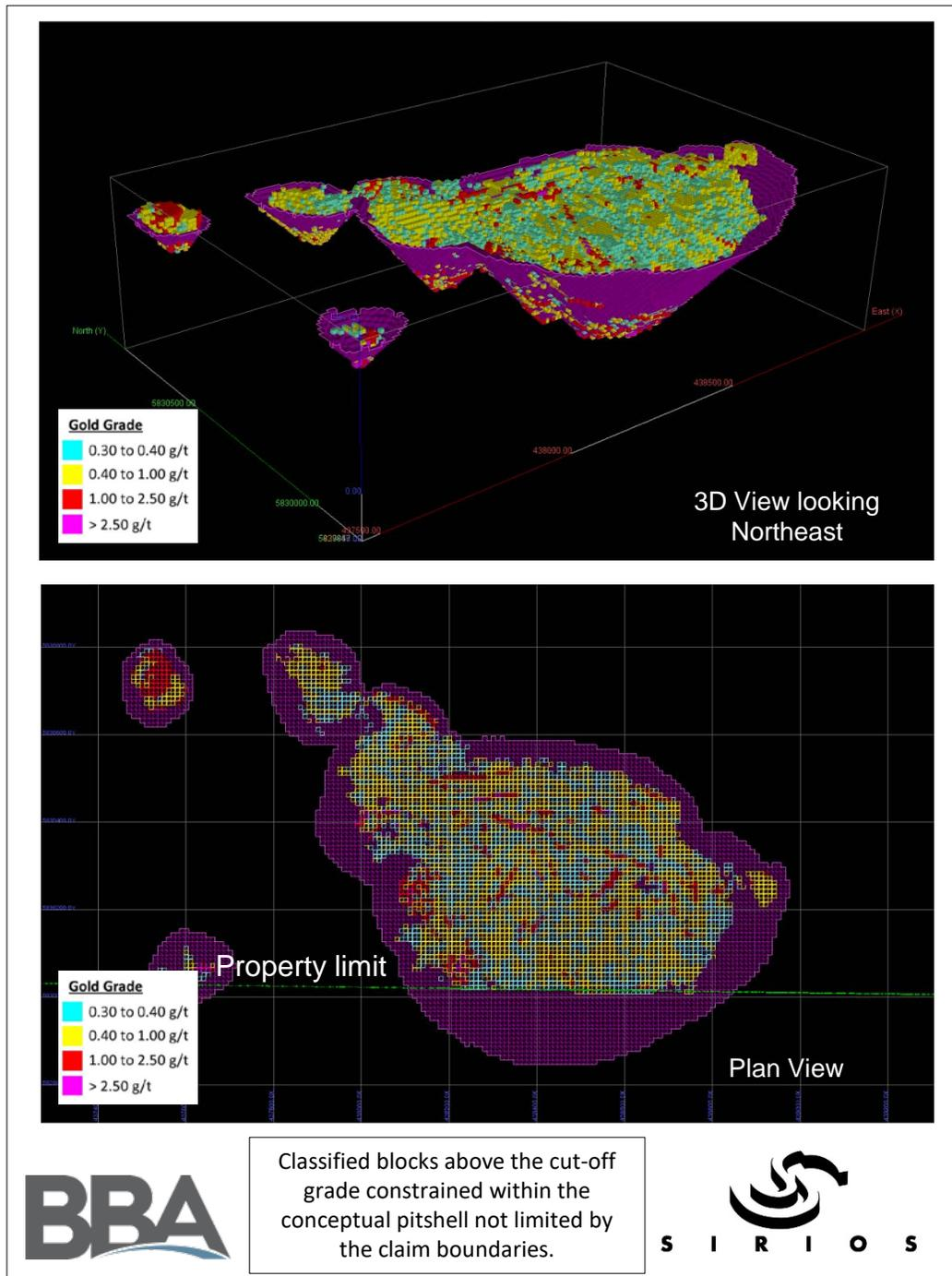
Figure 14-24: 3D and plan views showing grade distribution and classification of the Project above the cut-off grade
