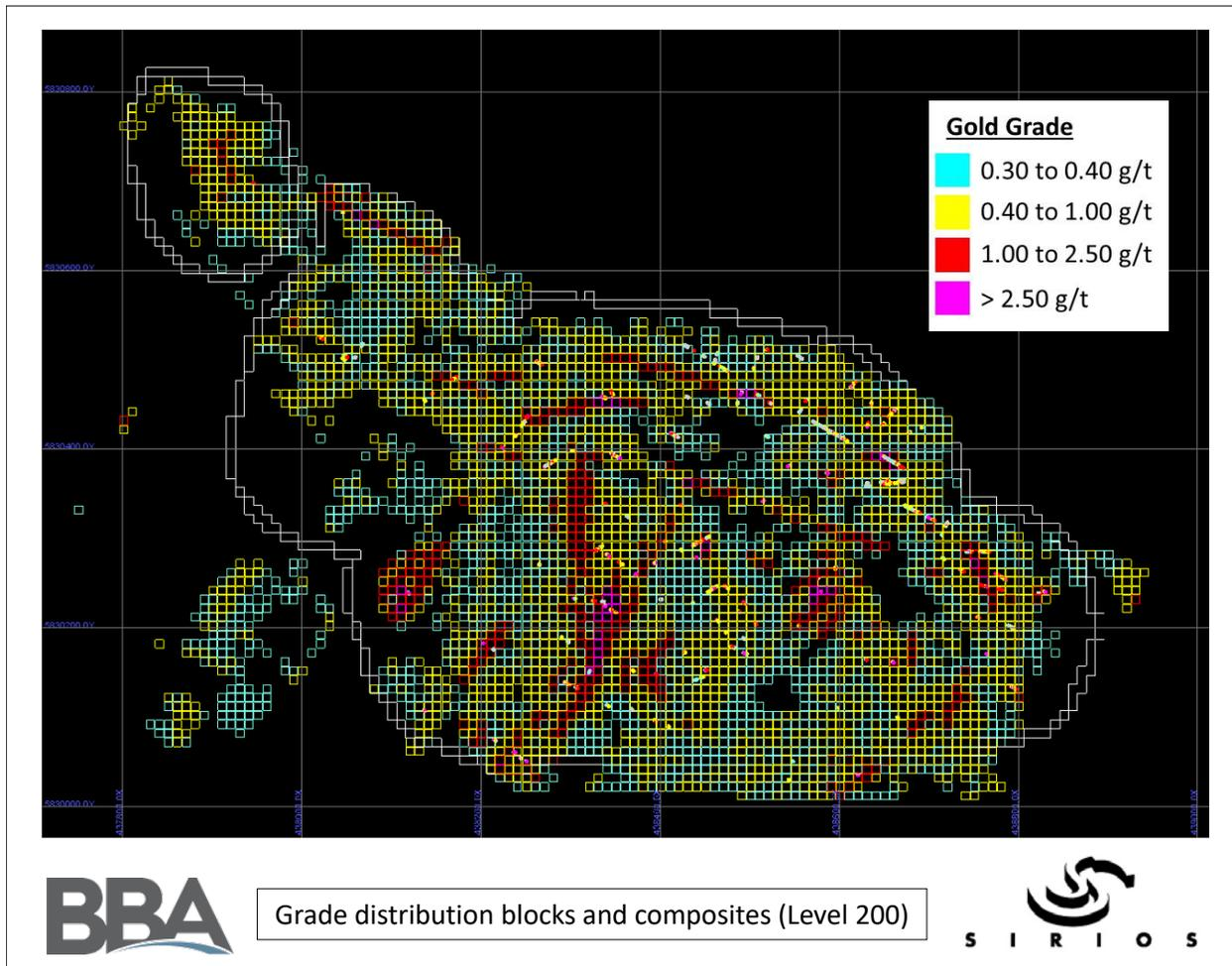
**Figure 14-17: Comparative example of the grade distribution between the blocks and the composites in plan view (Level 200)**
