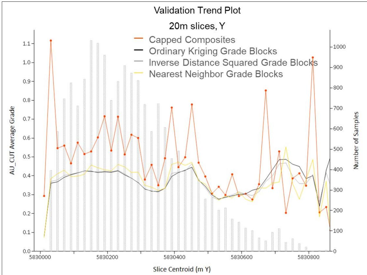
Figure 14-19: Block model validation swath plots across strike (Y-direction)
