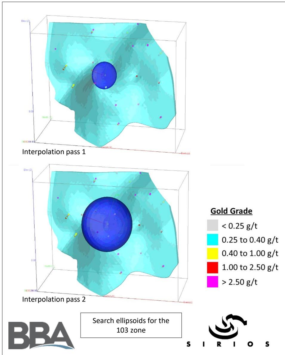
**Figure 14-15: Example of search ellipsoids for the 103 high-grade domain for the two interpolation passes**
