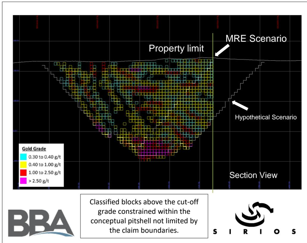
Figure 14-25: Section view showing grade distribution and classification of the Project above the cut-off grade
