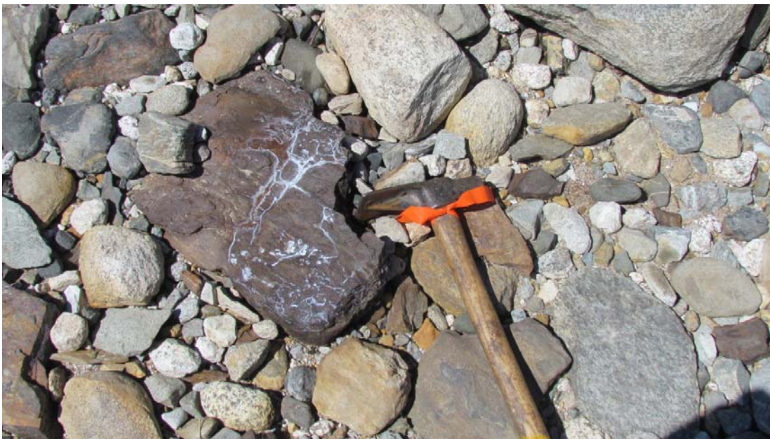
Picture 15: View of a boulder of pyrrhotite-bearing weathered amphibolites found in one of the boulder field along the shore of Opinaca Reservoir, about 1 kilometre down-ice of the Kasak Formation. White veinlets are jarosite or gypsum, sulfates from the oxidation of pyrrhotite. Assay result on this specific boulder is not known. Picture taken by the author.
