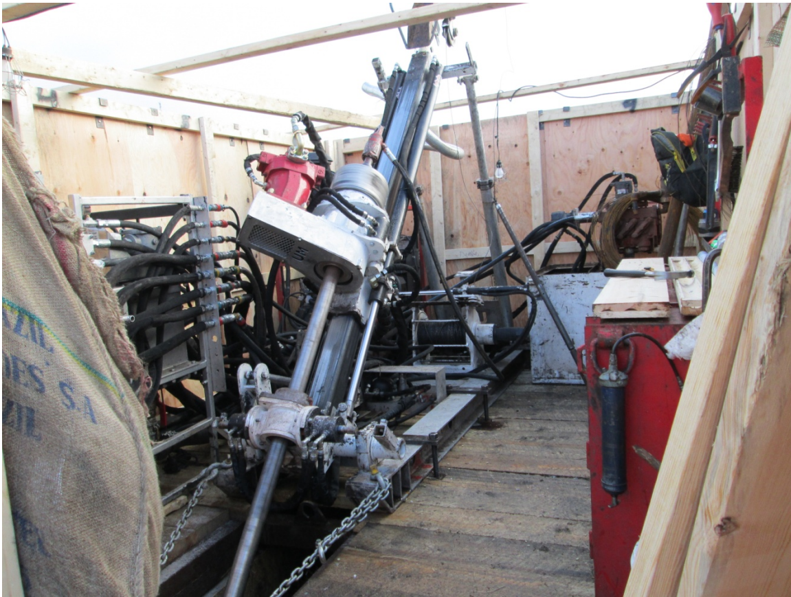
Picture 21: View of the Mancore drill used by G4 Drilling set in its plywood shack, ready to run.
