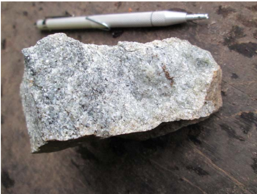
Picture 12: Detailed view of a trondhjemite sample mineralized by very fine arsenopyrite.
