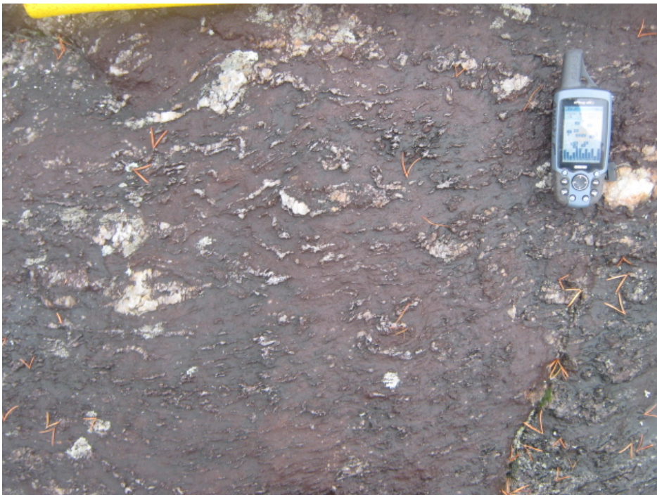
Picture 6: Sillimanite alteration affecting a paragneiss, a localized feature on Cheechoo-B-west.
