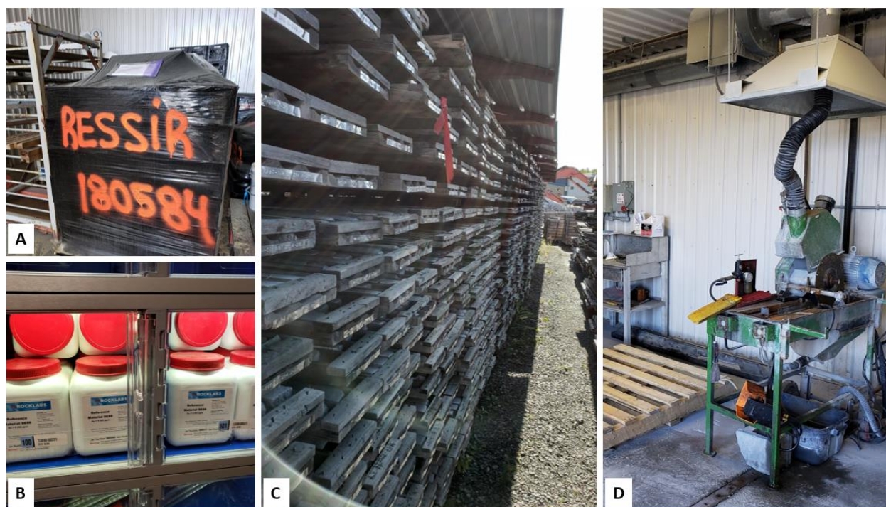
Figure 12-1: Storage and sampling procedures reviewed during the site visit at the Technominex facilities A) Wrapped drill core boxes; B) Properly stored CRM; C) Roofed drill core storage; D) Core saw used to sample the core
