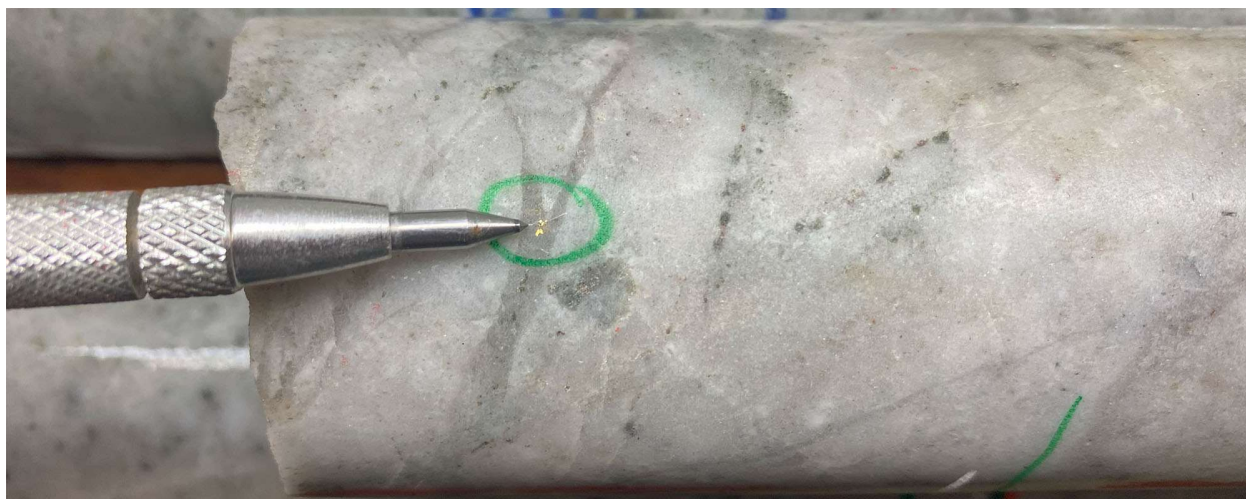
Figure 4.5: CH24-317, 189.0 m: Visible gold in quartz stockwork with arsenopyrite.
