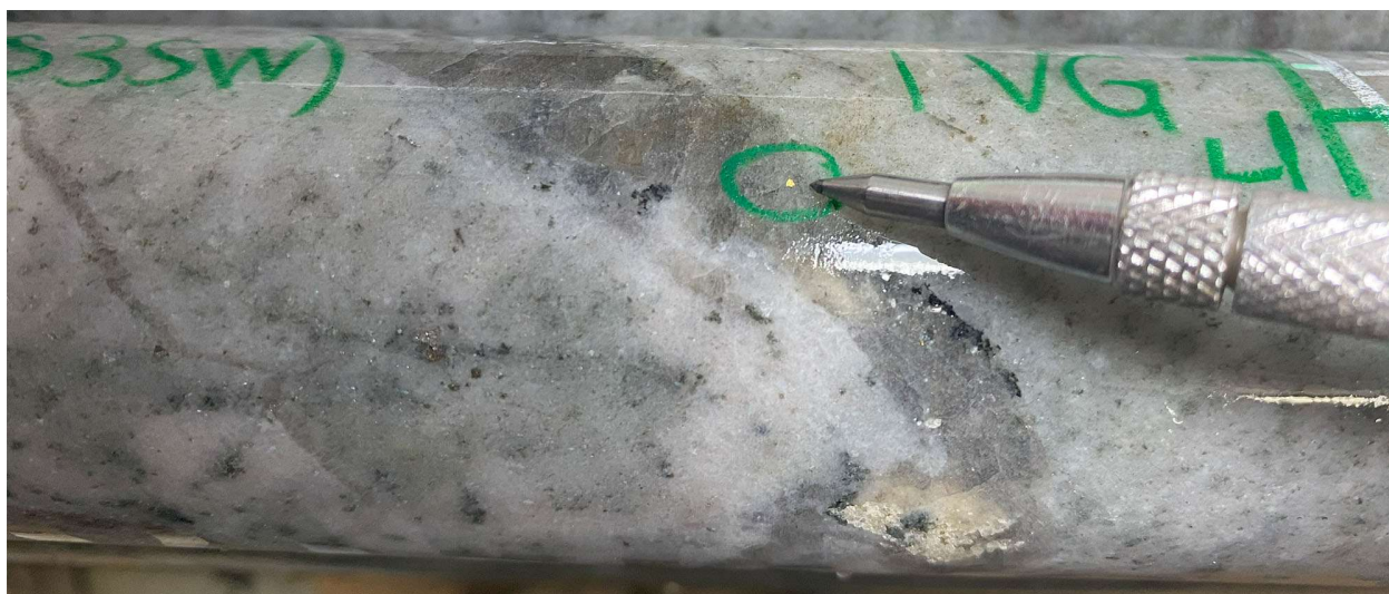
Figure 4.4: CH24-317, 178.3 m: Visible gold in a quartz veinlet with arsenopyrite and scheelite.
