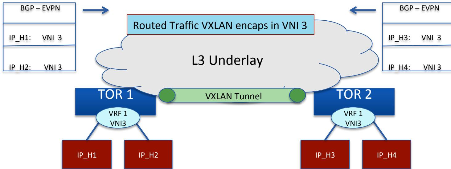
Advertisement of IP:VNI bindings from a TOR via BGP EVPN enables a remote TOR to send routed traffic to that IP using the VNI for that IP to the TOR that advertised the IP over VXLAN
