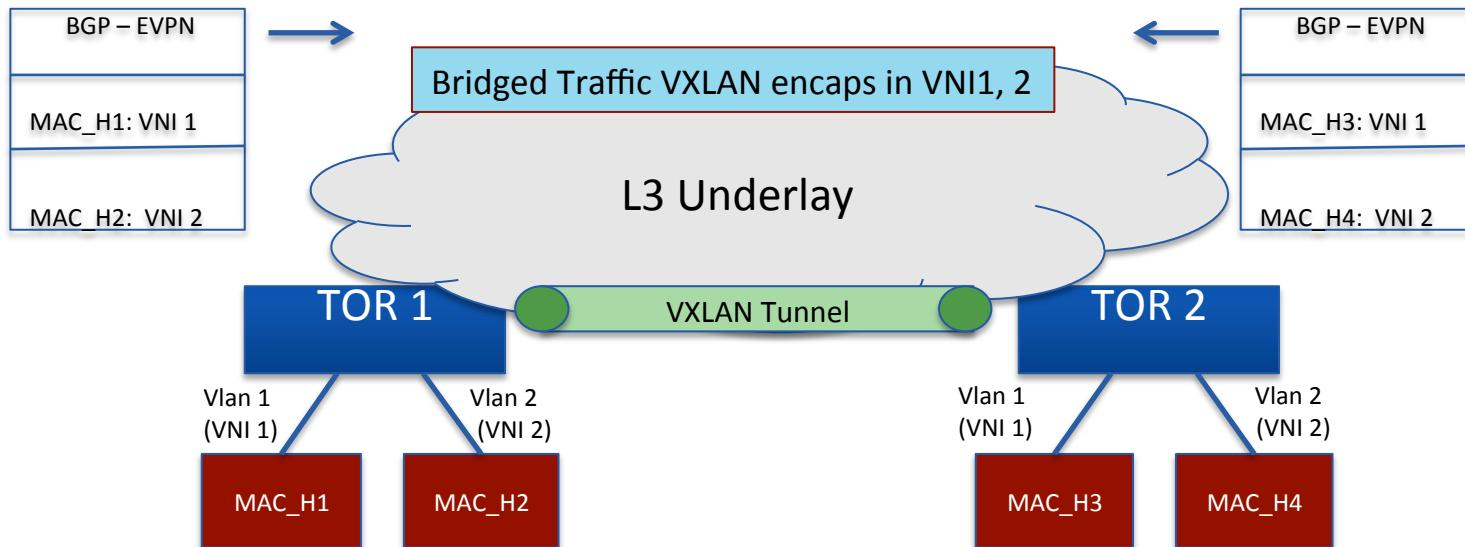
Advertisement of MAC:VNI bindings from a TOR via BGP EVPN enables a remote TOR to send bridged traffic to that MAC using the VNI for that MAC to the TOR that advertised the MAC over VXLAN
