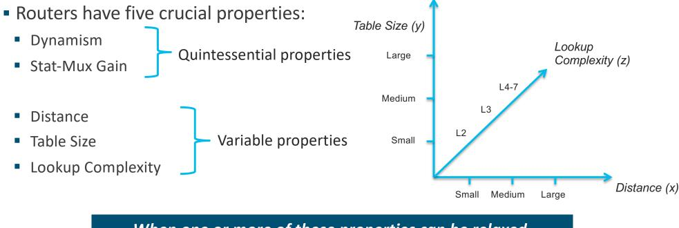
When one or more of these properties can be relaxed, a router can be delivered of lower cost.
