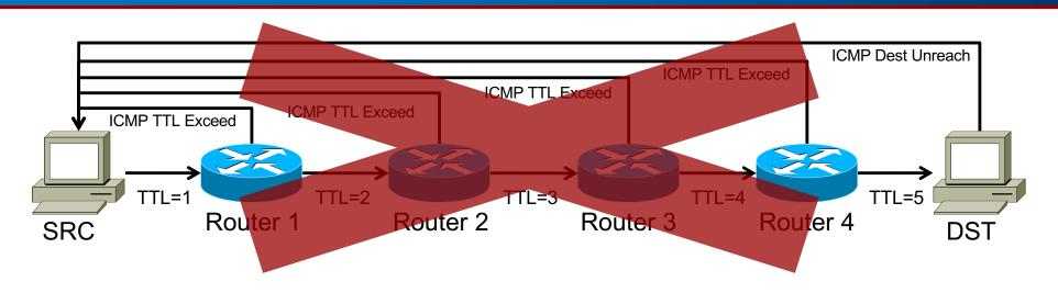
All returned ICMP packets must travel to the end of the LSP before going back to the sender. This makes every hop in the LSP appear to have the same RTT as the final hop.
