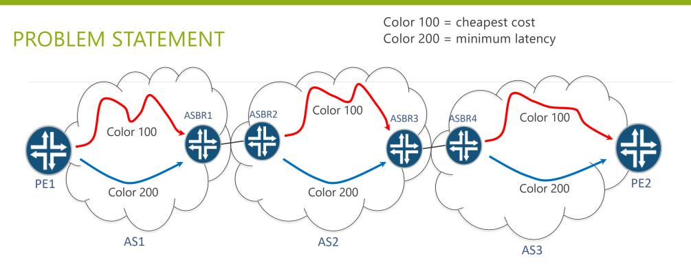
PE1 wants to send traffic to PE2 in another AS using colored transport. It can reach the local ASBR, ASBR1, using the preferred color of transport.
