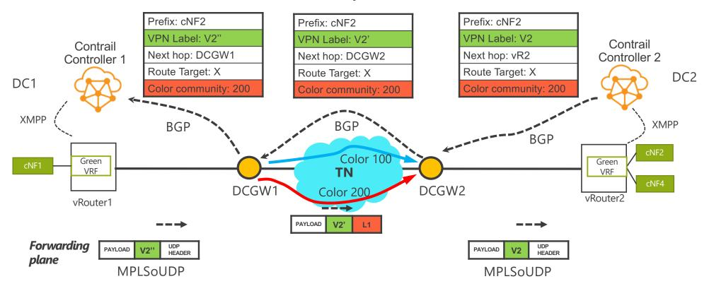
Key point: DCGW1 puts the traffic for cNF2 onto the Flex-Algo or TE-LSP that has color 200, because the BGP prefix has color community 200.
