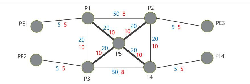
Normal IGP metric in blue font. Bulk traffic uses the *normal IGP*. IGP metrics are configured so that the traffic tends to use the high bandwidth links.
