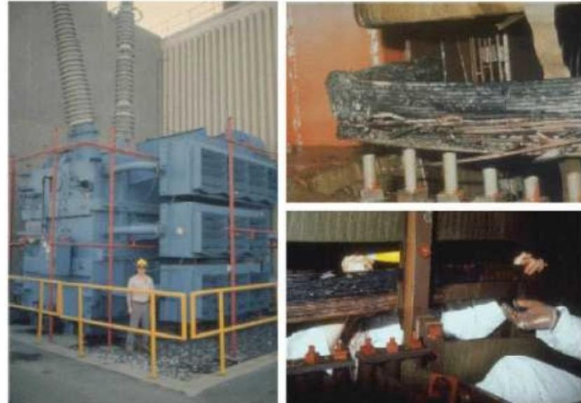
Heating so intense insulation was burned away and wires melted together
