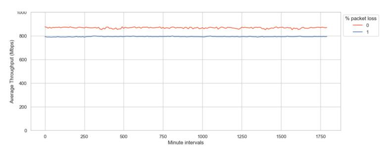
On average, **1%** of packet loss caused **8.5%** decrease in throughput while using BBR, stark difference to **70.7%** decrease using CUBIC!
