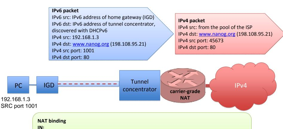
IPv6 src: IPv6 address of IGD + 192.168.1.3 + port1001
