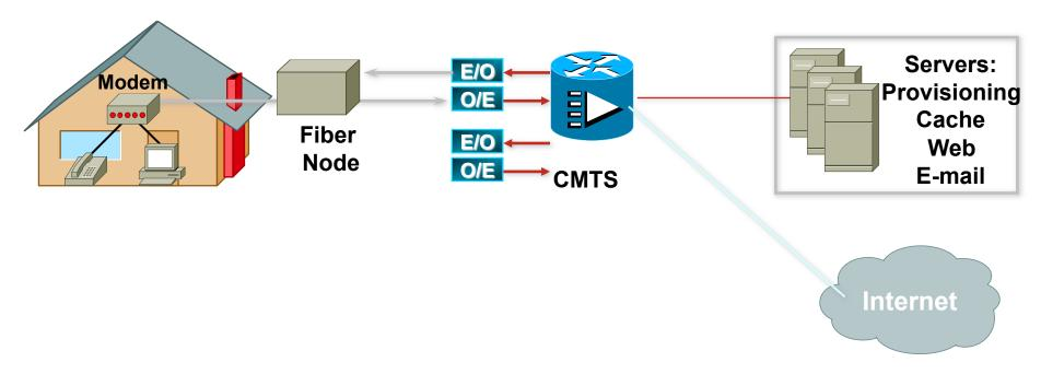
Note: E/O and O/E refer to the Electrical to Optical conversion of the signals in a cable HFC system
