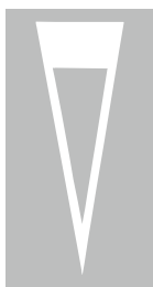
Warning of 'Give Way' just ahead
