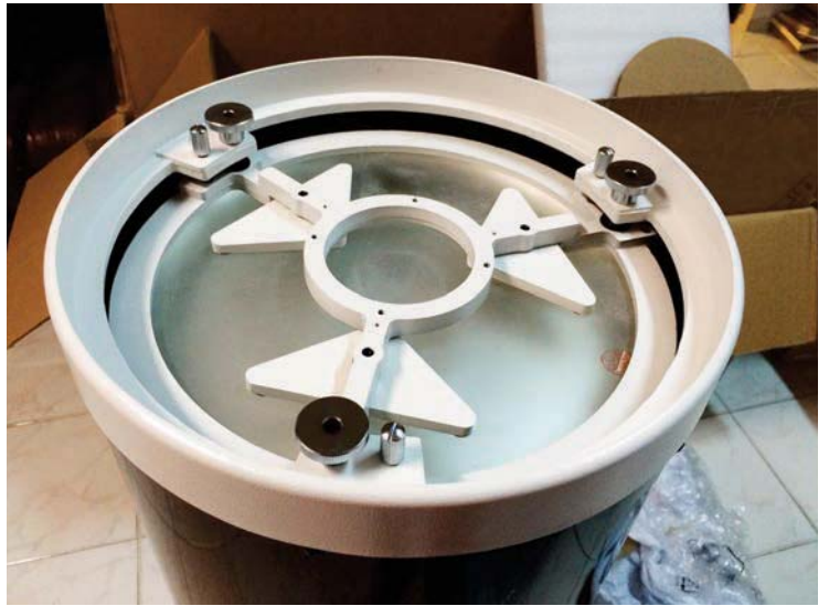
Image 5 - Mirror cell from the back.
