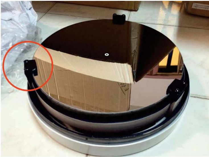
Image 4 - Don't over tighten!
