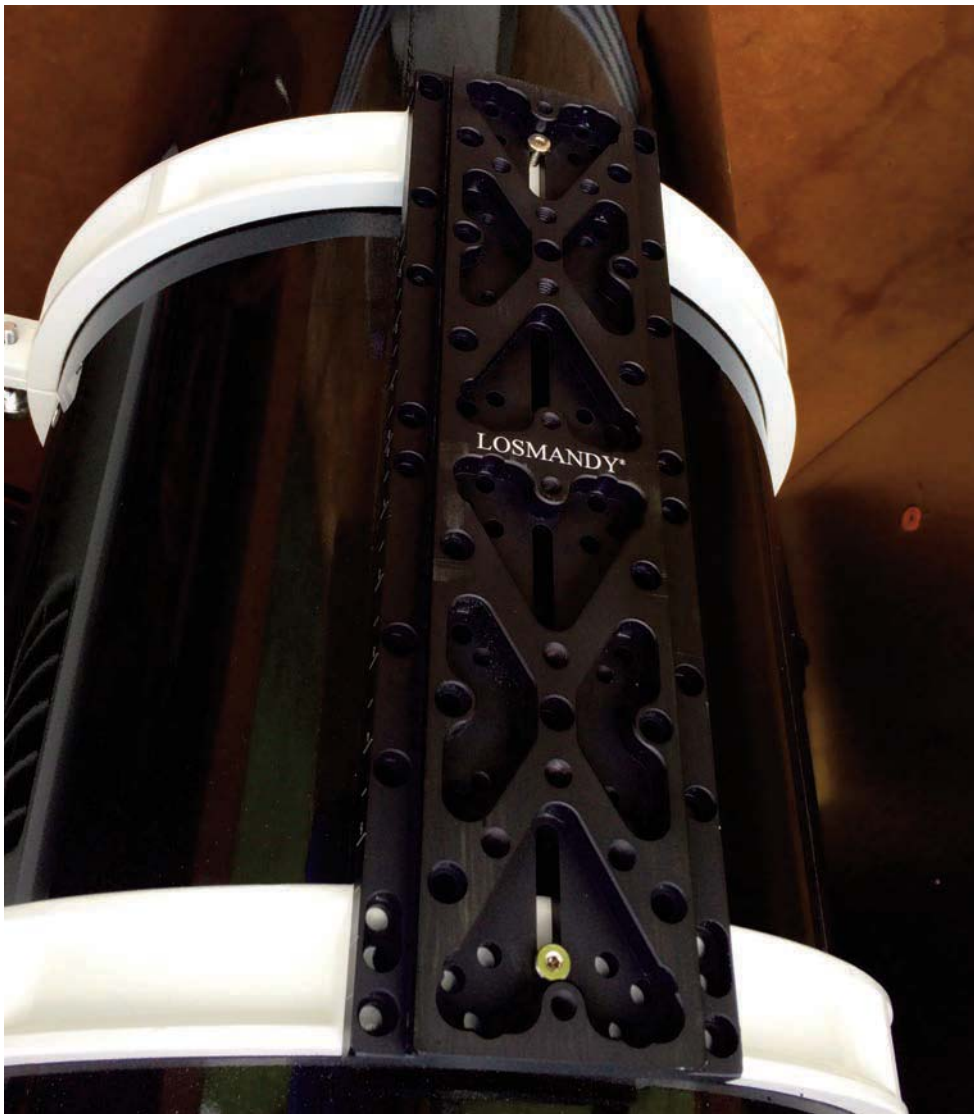
Image 7 - A retrofit to the dovetail as needed for my mount's Losmandy D-style connection.
