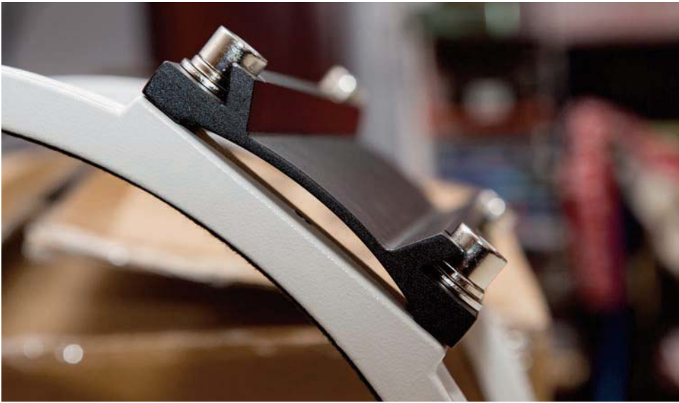
Image 6 - Protruding bolts prevented sliding into the versa-plate.
