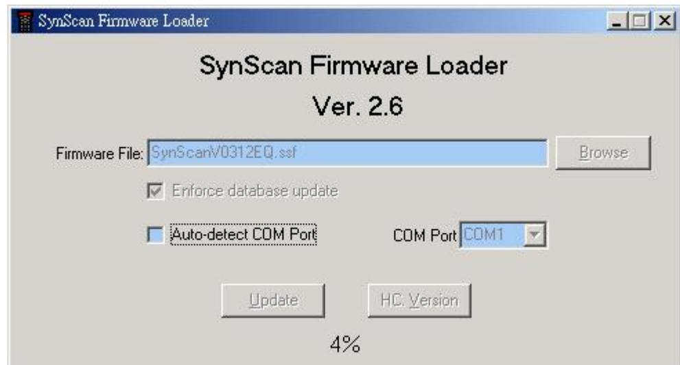
6. When the download is complete, a green “Update Complete” bar will show at the bottom of the Firmware Loader (Fig.x). The SynScan hand control is now updated to the newest firmware. Generally it takes about 1 minute to update the firmware. It may take longer if you are using an USB to serial converter.
