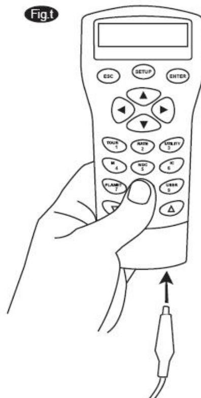
Manual). Push the connector into the hand control until it clicks into place. Plug the other end of the cable, the DB9 connector, to the RS-232 port on your PC.
