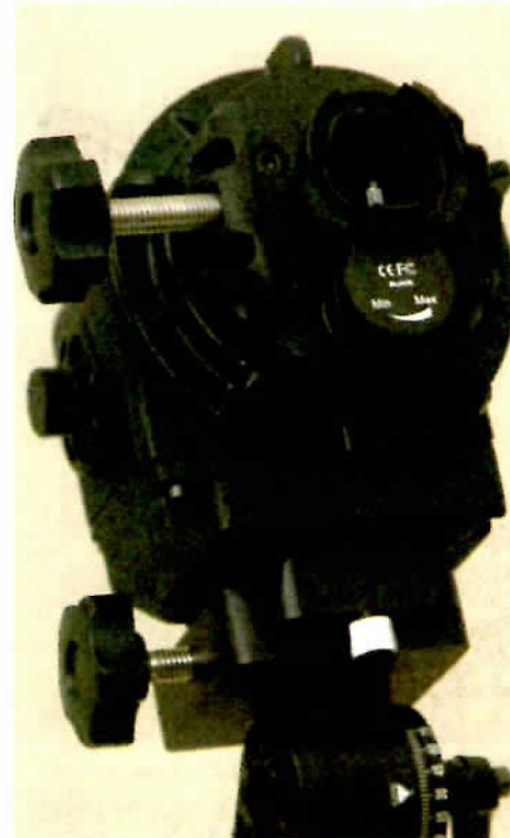
Image 7 - The kit includes a red-LED reticle illuminator, which presses into the front opening of the built-in polar-alignment scope
