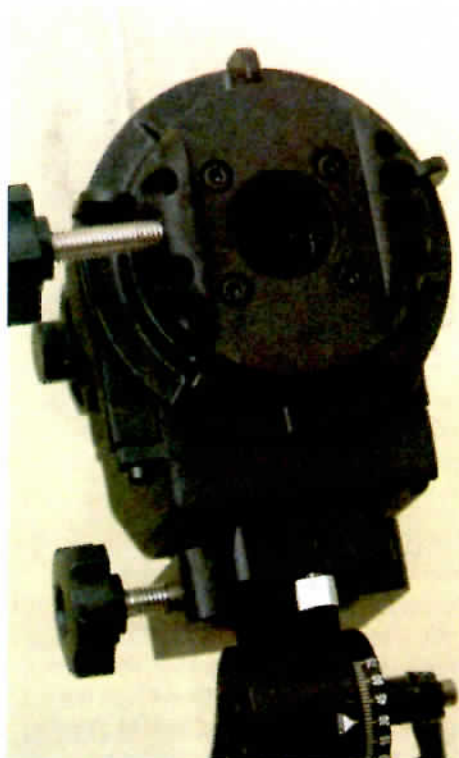
Image 5 - Removing a press-in cap reveals the front of the built-in polar-alignment scope.
