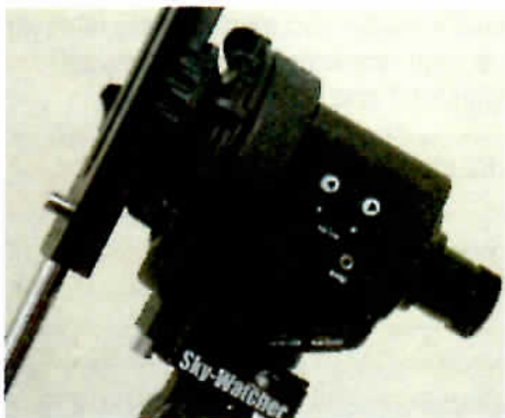
Image 9 - The left side of the mount features a mini-USB power port, and auto-guider port, a “snap” port for camera-shutter control, a switch for setting the mount to southern-hemisphere versus northern-hemisphere mode or for time-lapse mode, and left and right buttons.
