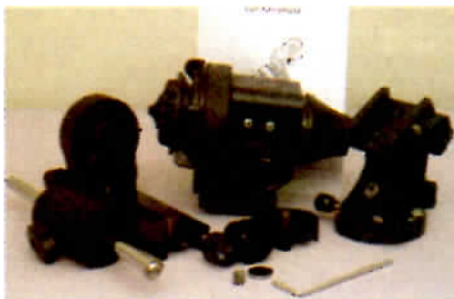
Image 16 -The collection of components that comprise the Star Adventurer Astro Package (plus counterweight kit).
