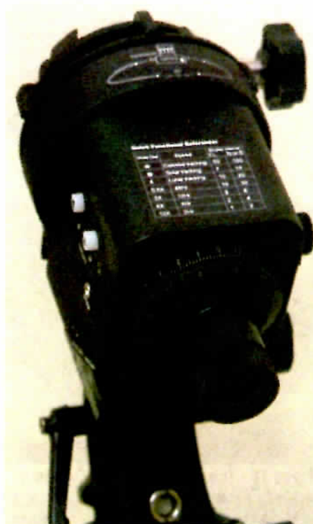
Image 6 - Removing a coned-shaped cover from the rear of the scope exposes the eye end of the polar-alignment scope.
