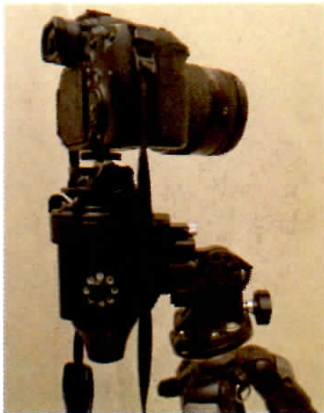
Image 13 - Although the equatorial wedge tops out at an altitude of 75 degrees, the northern tripod leg can be extended until the RA axis pointed directly at zenith for panning of time lapses along the horizon (Image 13). Weight the northern leg to keep the mount from tipping over.
