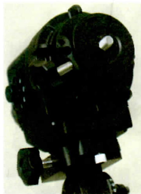
Image 12 - The included ball-head adapter allows replacement of the declination assembly with a standard camera ball-head mount.
