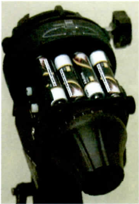
Image 8 - Four internal AA batteries are accessed by removing the snap-on cover from the top of the mount.
