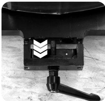
**3.3** Loosen the clamp until there is space enough to insert the support bar's ball ends.
