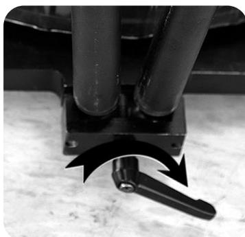
**3.4** Insert two support bars' ball ends into the groove (with corresponding #) and secure the clamp.
