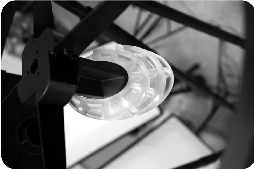
*A view of the cellular structure of the secondary flat mirror*
