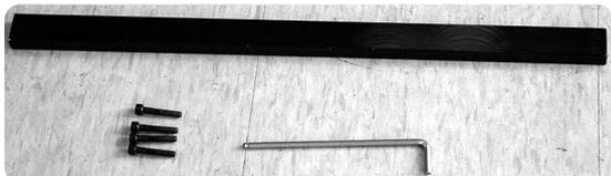
**5.5** Prepare the reinforcing bar and 4pcs M6x25mm Allen screws, and the 5mm Allen wrench.
