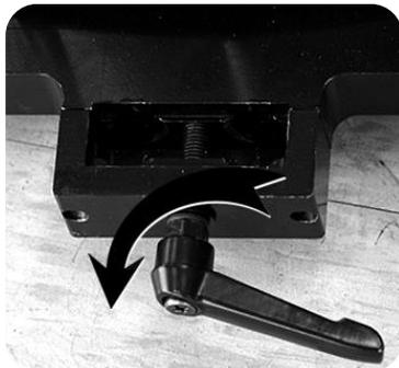
**3.2** Loosen the three clamps on the rear cell to pull the cover plate open.
