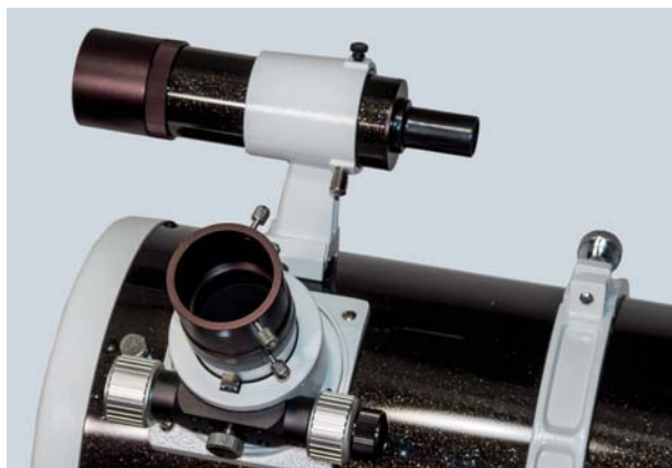
The Quattro line includes an excellent 9x50 finderscope attached with a standard dovetail shoe, which can be replaced with a 50-mm guidescope for autoguiding. The Crayford-style focuser comes with adapters for 1¼- and 2-inch eyepieces. The 2-inch adapter is shown here.
