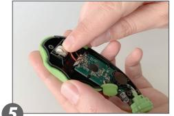
Insert 3 new L1154F batteries into gauge with positive side facing the top of the gauge. Gauge will turn on when inserted correctly.
