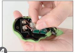
Remove old batteries from gauge being careful not to break small battery contact wires.
