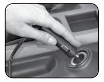
Switch inflator "On," and inflate tire to manufacturer's recommended air pressure. In passenger vehicles, this information can be found on the driver's side door jamb and owner's manual.
