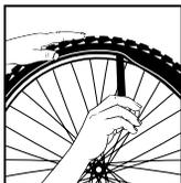
**6** Work other side of tire onto wheel being careful not to pinch the tube. A tire lever may be used if needed. Assure proper tire fit against rim.
