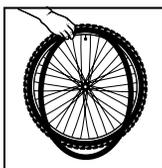
**5** Starting at the rim hole, insert valve and work tube onto the rim.
