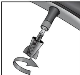
**6** Reinstall valve core.
