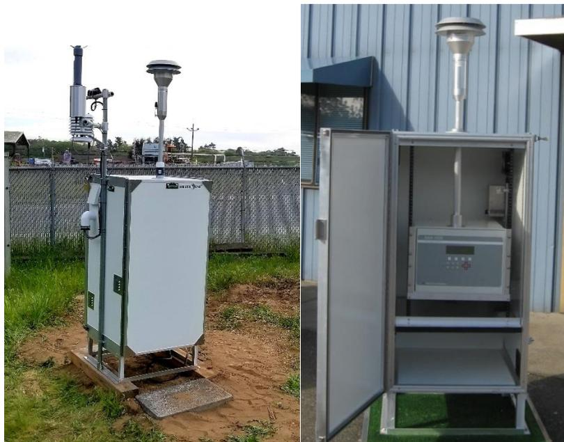
*Figure 2: The BAM 1020 PM<sub>10</sub> monitor in its enclosure.*
