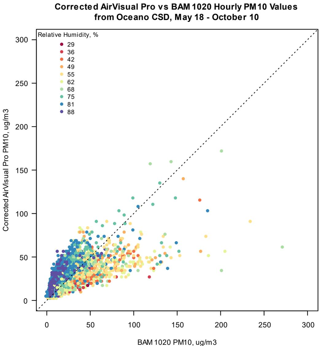
**Figure 11: Relative humidity effect on corrected BX-895 response.**
