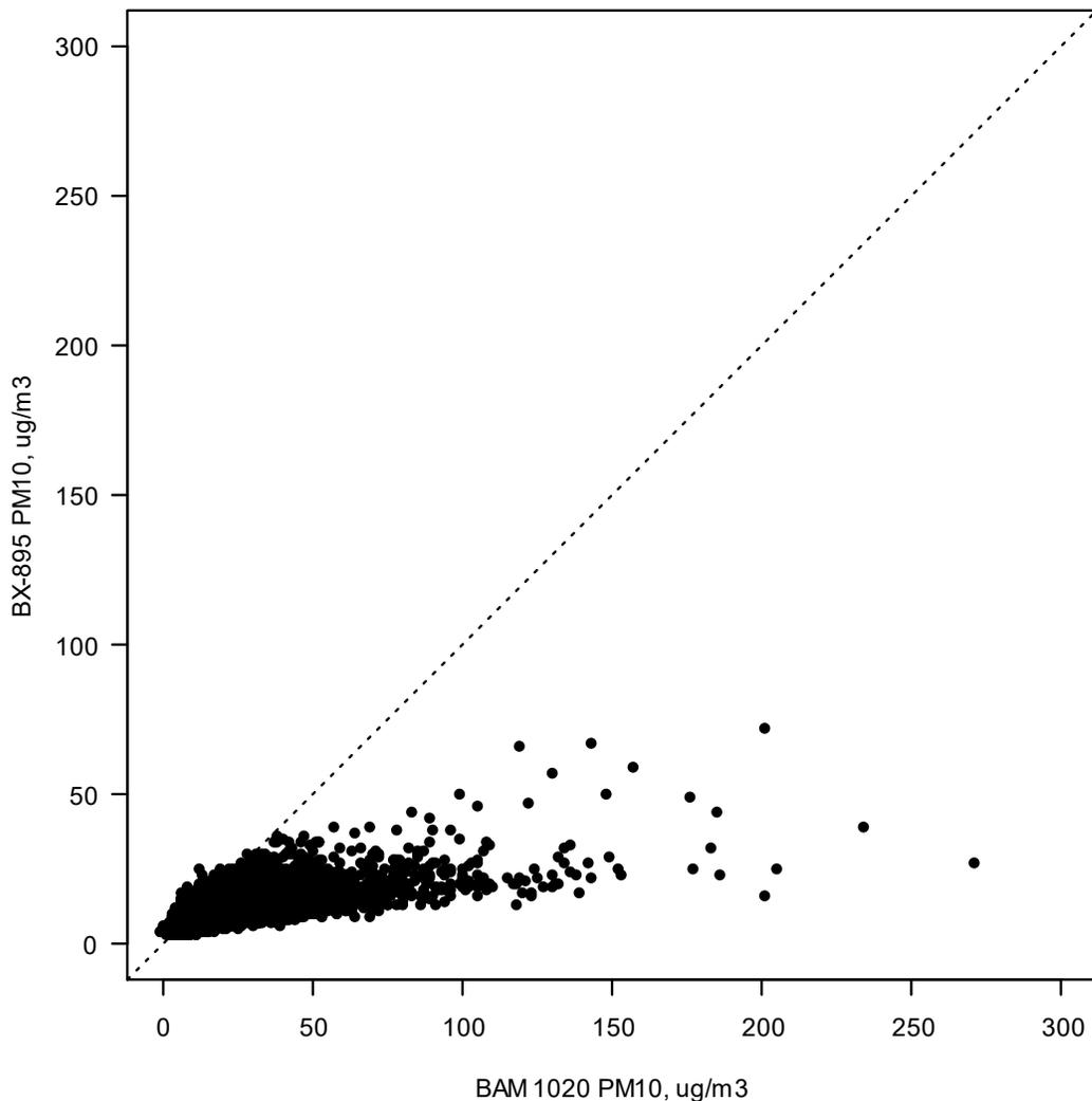
**Figure 10: Raw BX-895 PM<sub>10</sub> vs BAM 1020 PM<sub>10</sub> from Oceano CSD**
