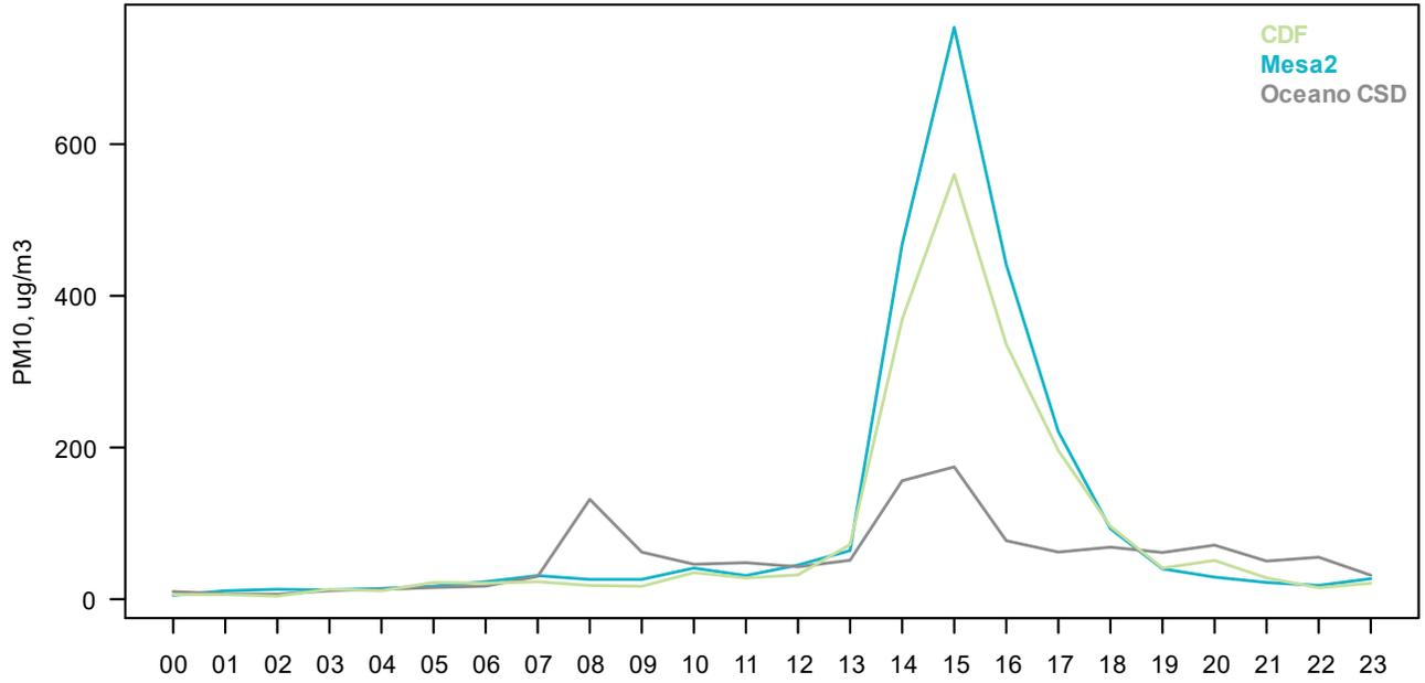
Figure 12: An example of hourly PM10 concentrations during windblown dust event.
