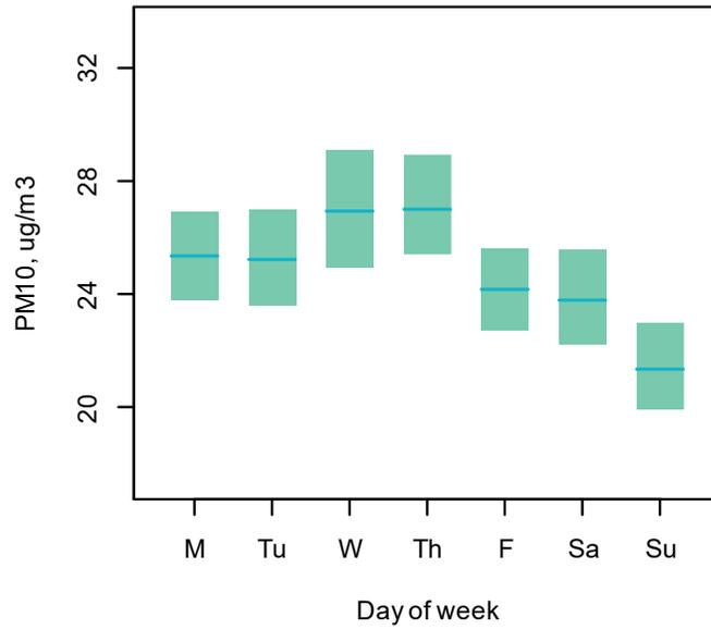
**Figure 16: Mean PM<sub>10</sub> at Oceano CSD by Day of the Week. 95% Confidence intervals shown in green.**
