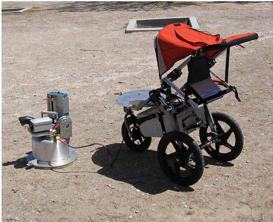
Figure 1. The current configuration of the PI-SWERL showing the cylindrical sampling chamber (left side of image) and the carriage used to transport it from site-to-site, which also holds the computer controlled data acquisition system.
