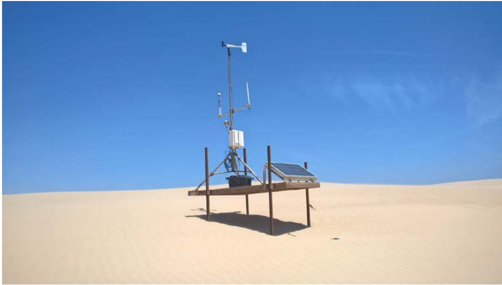
Figure 2-2. One of the 15 meteorological, saltation, and PM monitoring stations in the ODSVRA.
