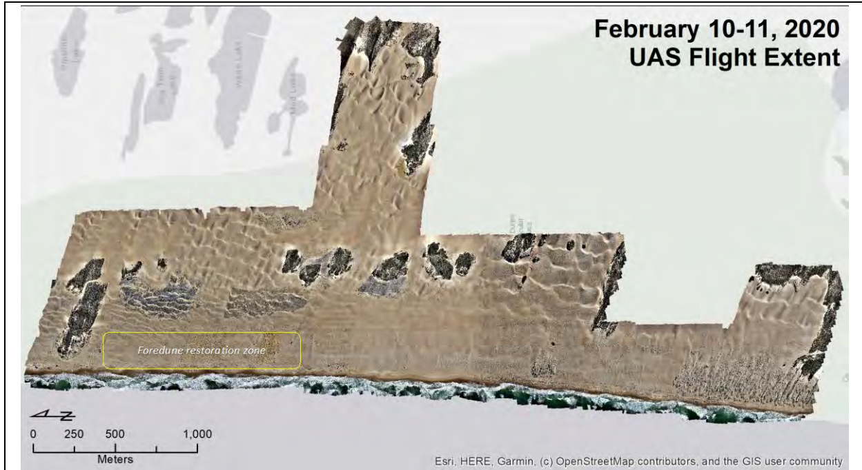
Figure 2-9. Orthophoto mosaic showing the approximate extent of the expanded UAS DEM mapping domain derived from February 2020 imagery collected by ASU. General area of the foredune restoration zone shown by the yellow polygon. Further details in Attachment 5.
