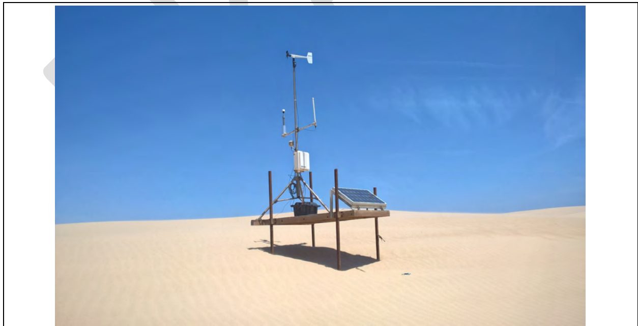
Figure 2-2. One of the 15 meteorological, saltation, and PM monitoring stations in the Oceano Dunes SVRA.
