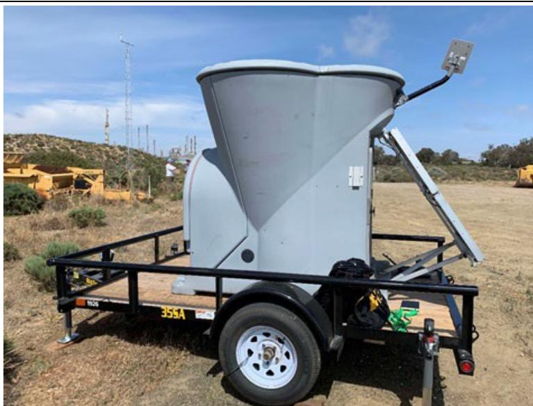
**Figure 2-5.** The SODAR upper-air measurement station is located near the southeast corner of ODSVRA. The photo shows the co-located 10-meter meteorological tower and the Phillips 66 refinery in the back left. UCSB and ASU operate the station.
