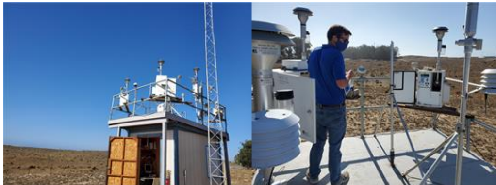
Figure 2. The Partisol samplers and BAM 1020 monitors at the CDF sampling site. All sampler inlets (Partisols and BAMs) were approximately 4.0 m above ground level (Photo credit, David Cardiel).
