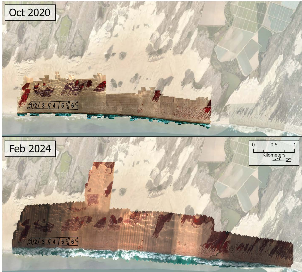
Figure 5. Multispectral false-color (G+B+NIR) UAS orthomosaics captured from a Micasense RedEdge-MX 5-band sensor (R, G, B, RE, NIR) in Oct. 2020 and a Micasense RedEdge-P 6-band sensor (R, G, B, Pan, RE, NIR) in Feb. 2024, used to map vegetation cover. Contrast differences are only visual and do not impact the indices calculated from the values of compared bands. Locations of the FRA treatment plots are outlined.
