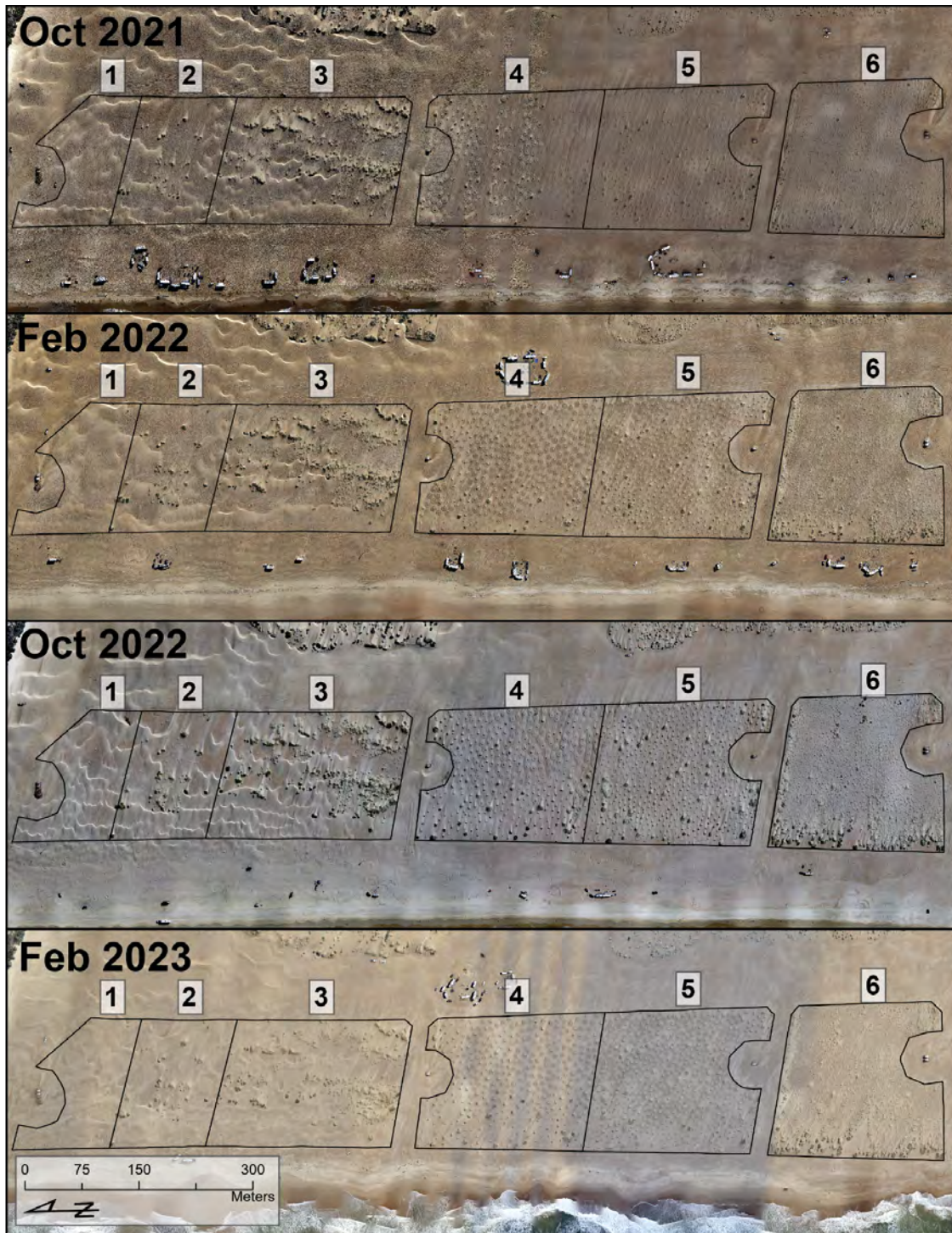
Figure 5. Foredune treatment plots from the second four visible (RGB) UAS mapping campaigns (Oct. 2021, Feb. 2022, Oct. 2022, Feb. 2023). Numbers correspond to the following restoration treatments: 1) Sheepsfoot texturing only (control site), 2) native seeds, 3) native seeds + sterile
