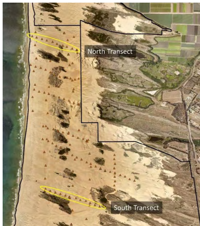
Figure A_1: PI-SWERL measurement transects used to assess potential west-east trends. Only the data points from 2013 are represented, but virtually identical locations were sampled again in 2015 and 2019.
