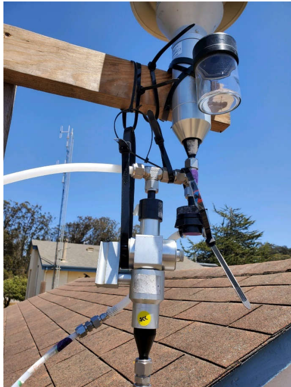
Figure 2: Scripps's PM_{10} sampling setup for 2021. Note the T fitting between the PM_{10} head and the sample holder. The split-off flow is further split by a second T before a portion is run through an SCC.
