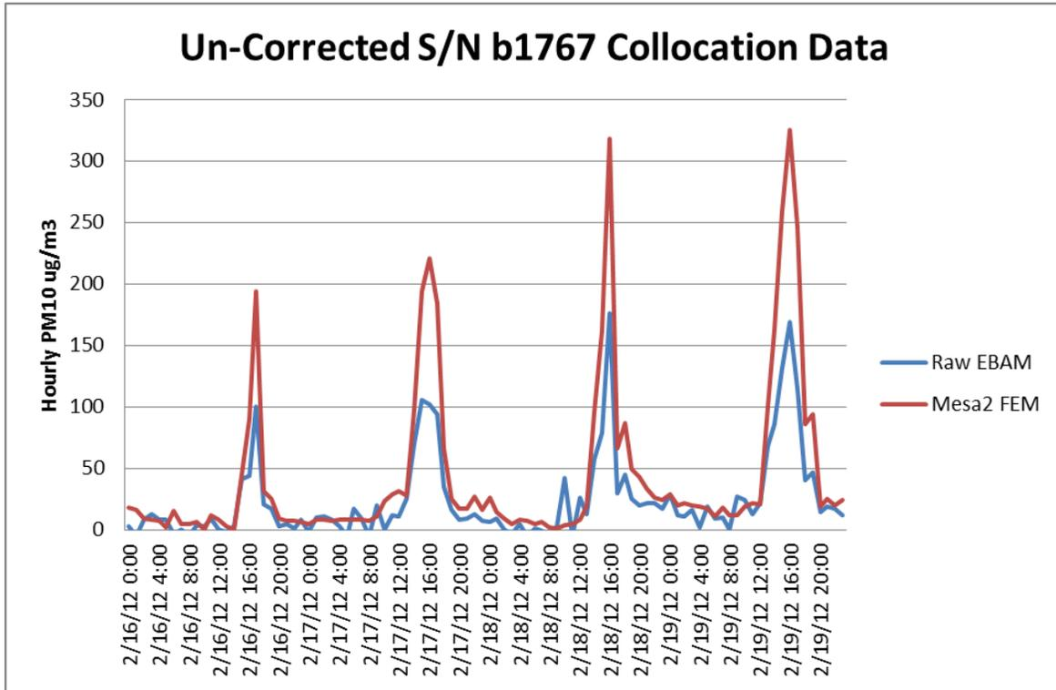
Figure A9 – Uncorrected EBAM S/N b1767 Data Compared to Mesa2 FEM
