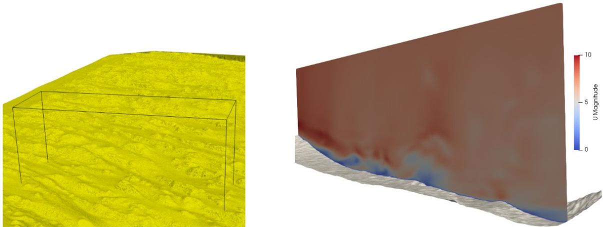
**Figure A. Left:** An example of a small computational domain placed over the Oso Flaco topography. **Right:** An example of velocity magnitude pattern across a portion of the dune from a preliminary simulation inside the domain.
