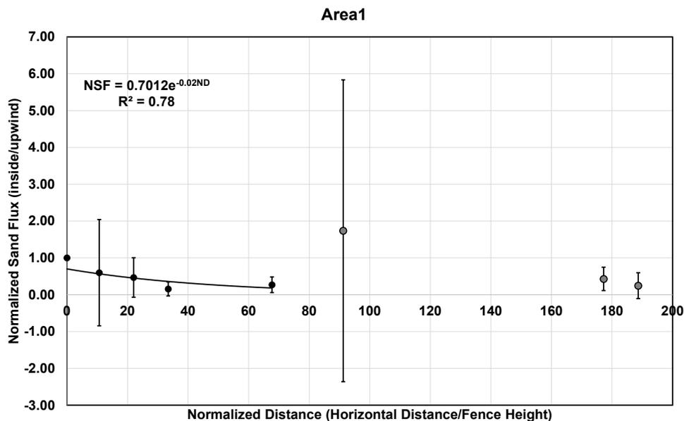
**Figure A.** Mean normalized sand flux as a function of normalized distance for the fence array Area 1 in 2020. The regression represents the change in NSF as a function of ND between ND 0 to 66.7 (black circles).
