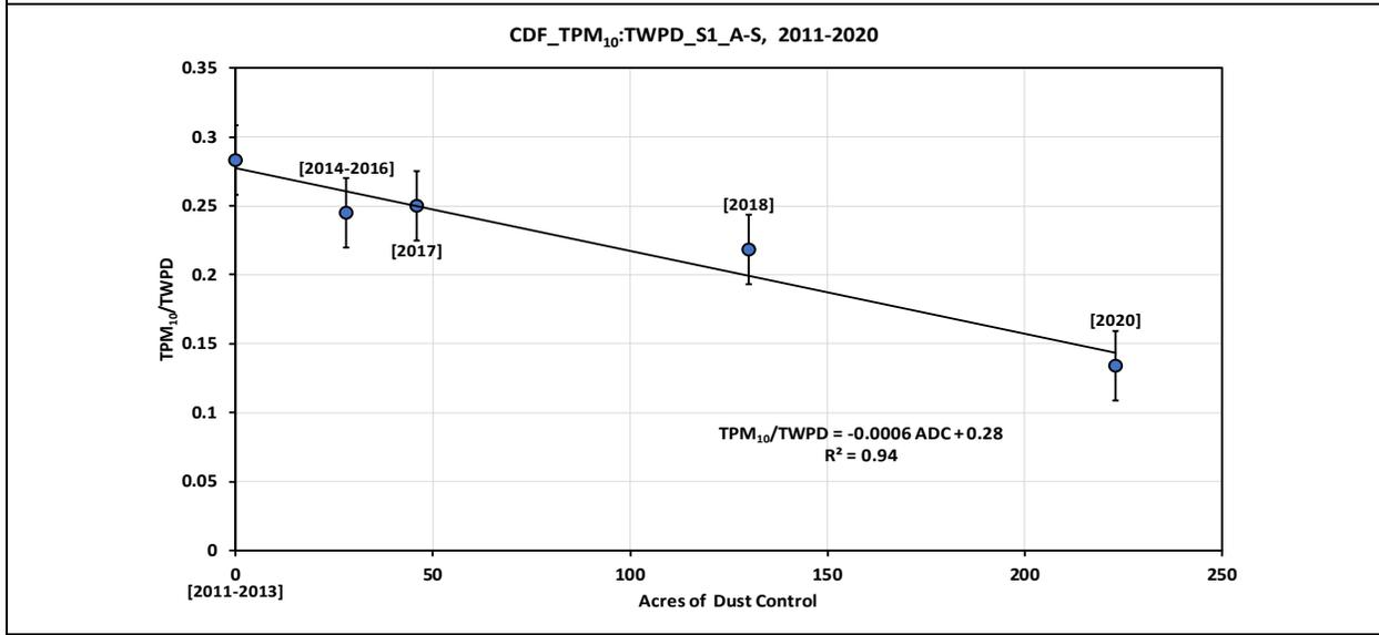
The relationship between the TPM<sub>10</sub>: TPWD ratio and acres of dust control for CDF total PM<sub>10</sub> data and the S1 total WPD data from 2011-2020 for the April through September period. Dates for the amounts of acres of dust control are shown in parentheses, and the error bars represent the Standard Error (std d/(#obs-1)<sup>0.5</sup>).
