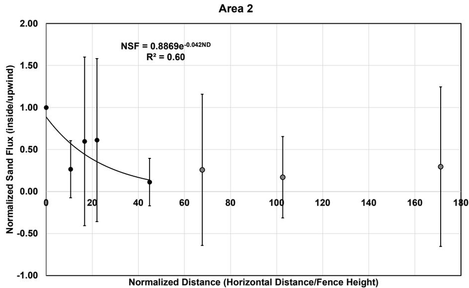
**Figure B.** Mean normalized sand flux as a function of normalized distance for the fence array Area 2 in 2020. The regression represents the change in NSF as a function of ND between ND 0 to 44.9 (black circles).
