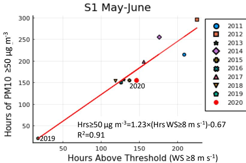
**Figure 4.** Total hours of PM<sub>10</sub> ≥ 50 μg m<sup>-3</sup> at CDF and total hours above wind speed ≥ 8.0 m s<sup>-1</sup> at S1 for the months May and June, 2011-2020.
