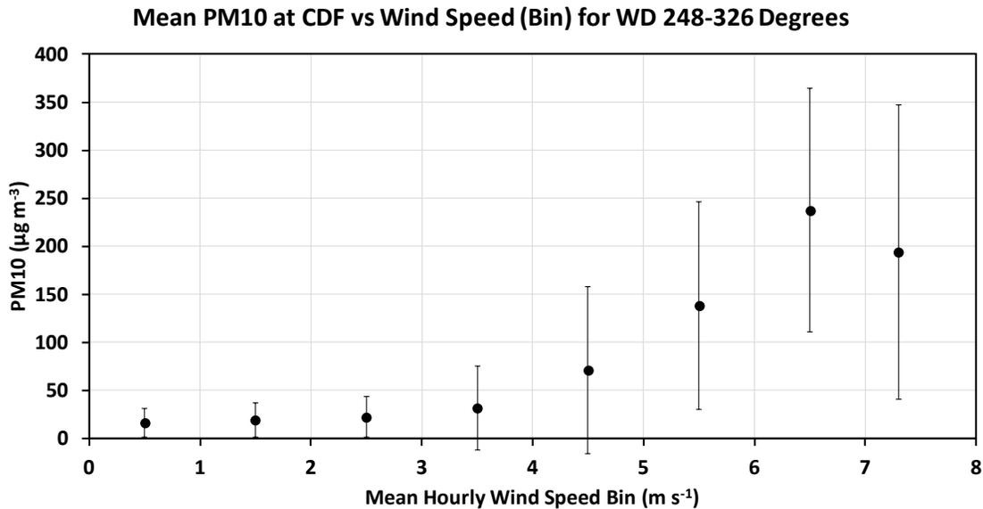
**Figure 1.** The relation between hourly mean PM<sub>10</sub> and hourly mean wind speed measured at 10 m AGL for winds from 248°-326° observed at the CDF monitoring station in 2019 (Jan-Dec). PM<sub>10</sub> increases as a function of wind speed bin for bins  $\geq 4.5$  m s<sup>-1</sup>.
