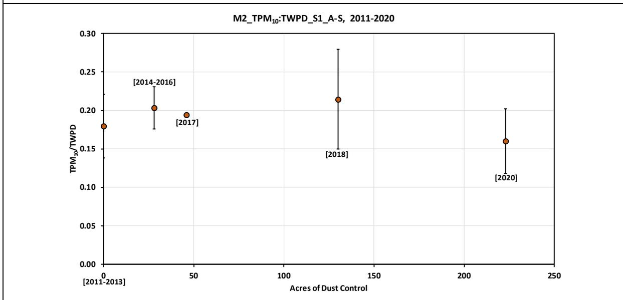
The relation between the TPM<sub>10</sub>: TPWD ratio and acres of dust control for Mesa2 from 2011 to 2020 (April through September). Dates for the dust control acreage are shown in parentheses, and the error bars represent the Standard Error.
