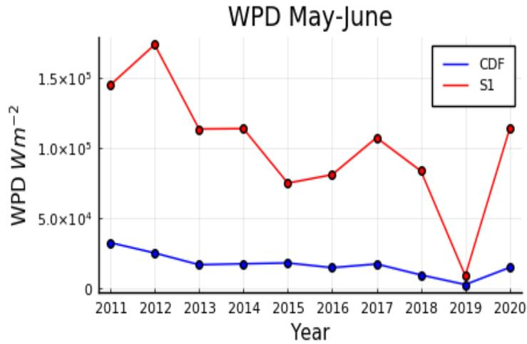
**Figure 5.** Total WPD ( $W m^{-2}$ ) for CDF and S1 tower (above threshold wind speed conditions), May and June, 2011-2020.
