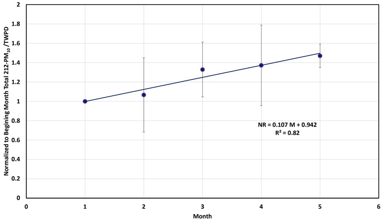
**Figure 17.** The mean normalized T212-PM<sub>10</sub>:TWPD ratio as a function of month-long increments of time. Data represent the period from May to September 2019 and include all in-Park stations (see Table 1). Note number on the X-axis does not represent month of the year, as the starting month for the normalization may be May or June.
