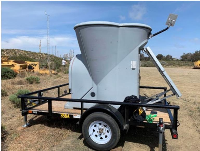
**Figure 2-5.** The SODAR upper-air measurement station is located near the southeast corner of Oceano Dunes SVRA. The co-located 10-meter meteorological tower and the Phillips 66 refinery are shown in the back left of the photo. UCSB and ASU operate the station.
