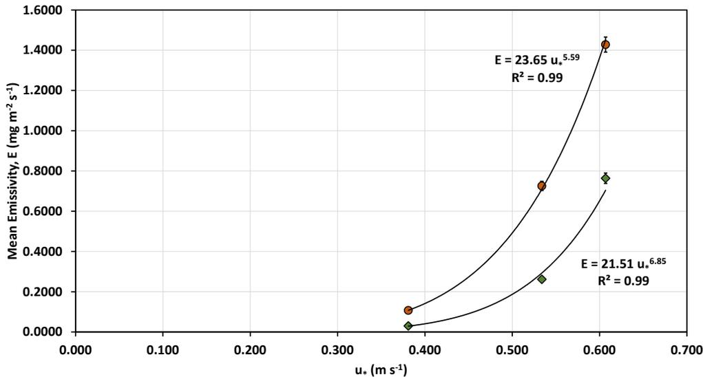
**Figure 3.** The relation between mean  $E$  ( $\text{mg m}^{-2} \text{s}^{-1}$ ) and  $u_*$  ( $\text{m s}^{-1}$ ) for the amalgamated data from 2013 to 2019 for the riding (orange circles) and non-riding areas (green diamonds). Error bars represent the standard error of the estimate (standard deviation/ $(\# \text{observations} - 1)^{0.5}$ ).
