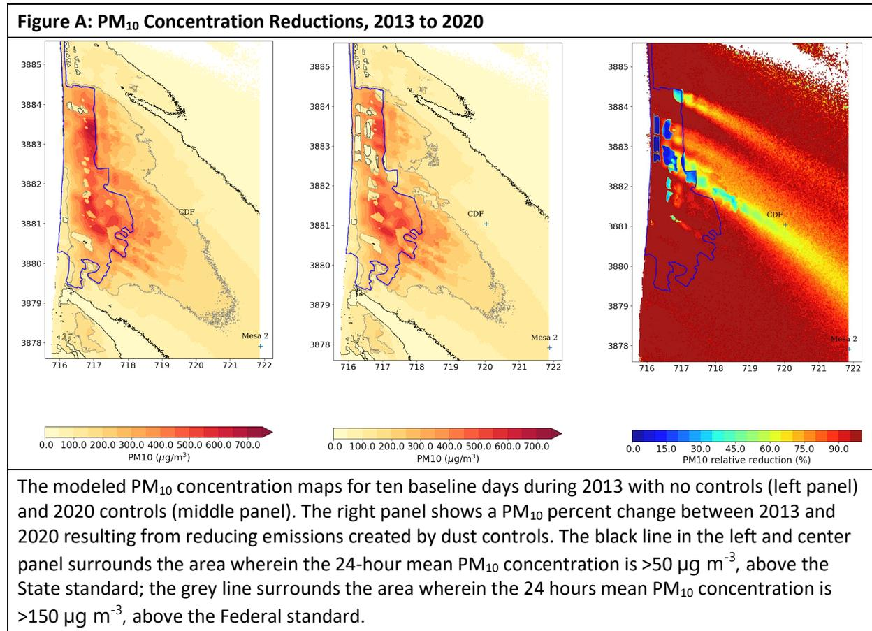
Measurements of PM<sub>10</sub> at CDF and wind speed at the S1 tower in Oceano Dunes SVRA are demonstrate that the dust emission system in locations where controls have been placed produces less PM<sub>10</sub> than prior to these controls. This reduction is consistent with the increase in acres of dust control. The analysis of observational data also converges with model results that indicate PM<sub>10</sub> reduction at the CDF receptor site is due to the dust controls.
