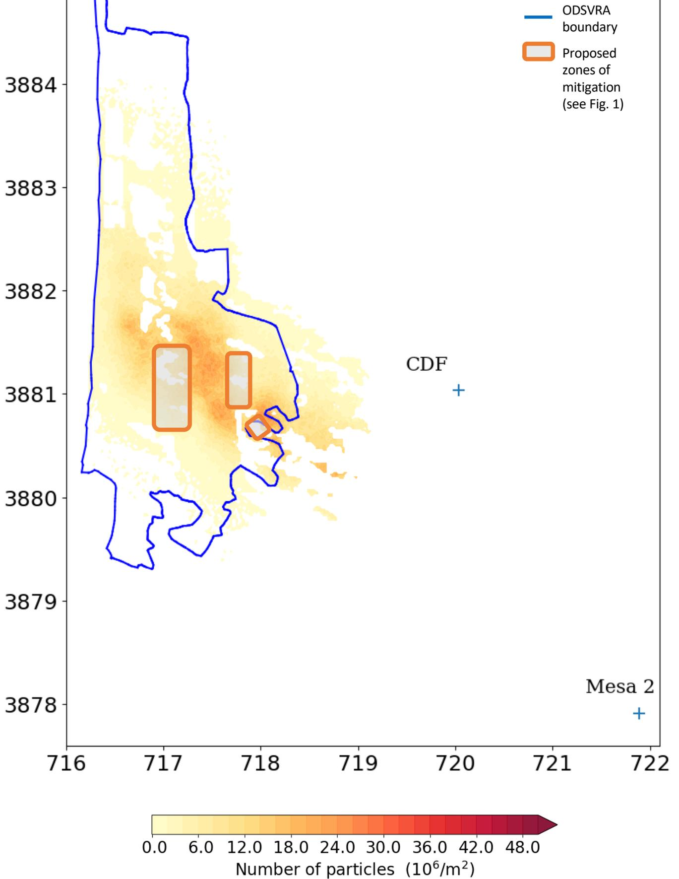
**Figure 3.** General locations of recommended dust mitigation treatments for the 2020-21 work plan shown overlain on the map of source attribution to the CDF monitoring station. Produced by DRI using 2013 data.
