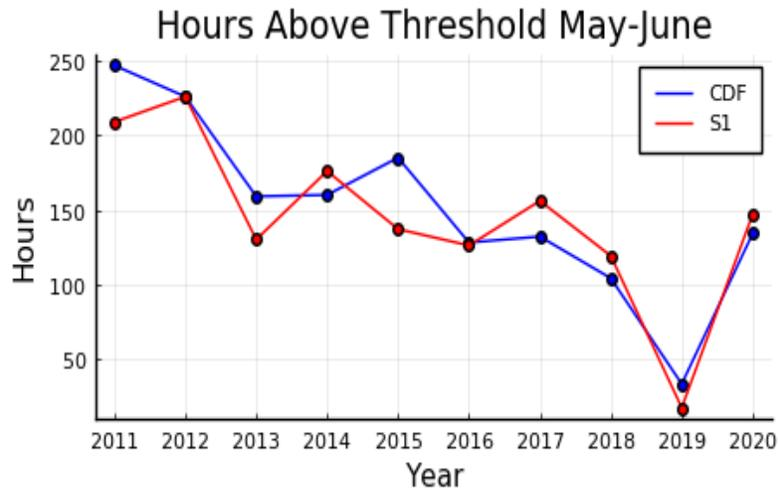
**Figure 2.** Total hours that wind speed is above the threshold of response for increasing  $PM_{10}$  at CDF (i.e.  $\geq 4.5 \text{ m s}^{-1}$ , 10 m AGL) and total hours wind speed is above the threshold of saltation at S1 (i.e.,  $\geq 8.0 \text{ m s}^{-1}$ , 10 m AGL).
