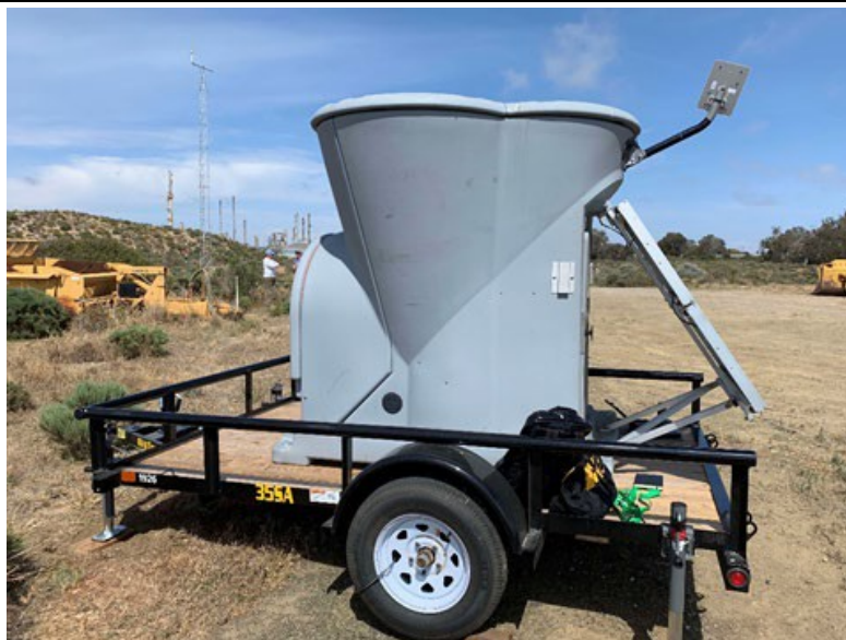
Figure 2-5. The SODAR upper-air measurement station is located near the southeast corner of ODSVRA. The photo shows the co-located 10-meter meteorological tower and the Phillips 66 refinery in the back left. UCSB and ASU operate the station.
