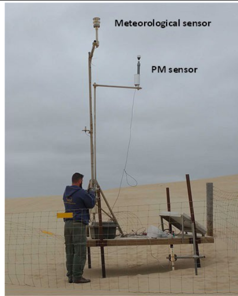
Figure 2-5. Typical meteorological (sonic anemometer) and PM (MetOne 212-2 Particle Profiler) monitoring site.
