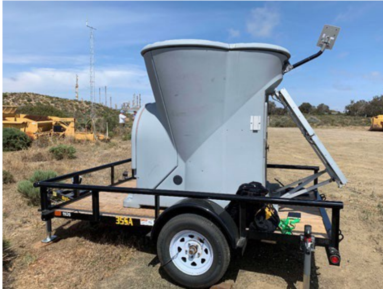
Figure 2-6. The SODAR upper-air measurement station is located near the southeast corner of ODSVRA. The photo shows the co-located 10-meter meteorological tower and the Phillips 66 refinery in the back left. UCSB operates the station.
