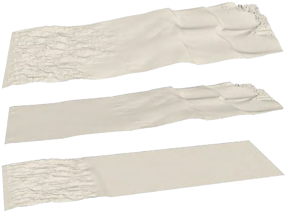
Figure 2: 3D representation of the topography of the mature Oso Flaco foredune test area (top panel) and two hypothetical geometry scenarios: the land surface with the foredune removed (middle panel), and the surface with a flat region behind the foredune with the transverse dunes removed (bottom panel).
