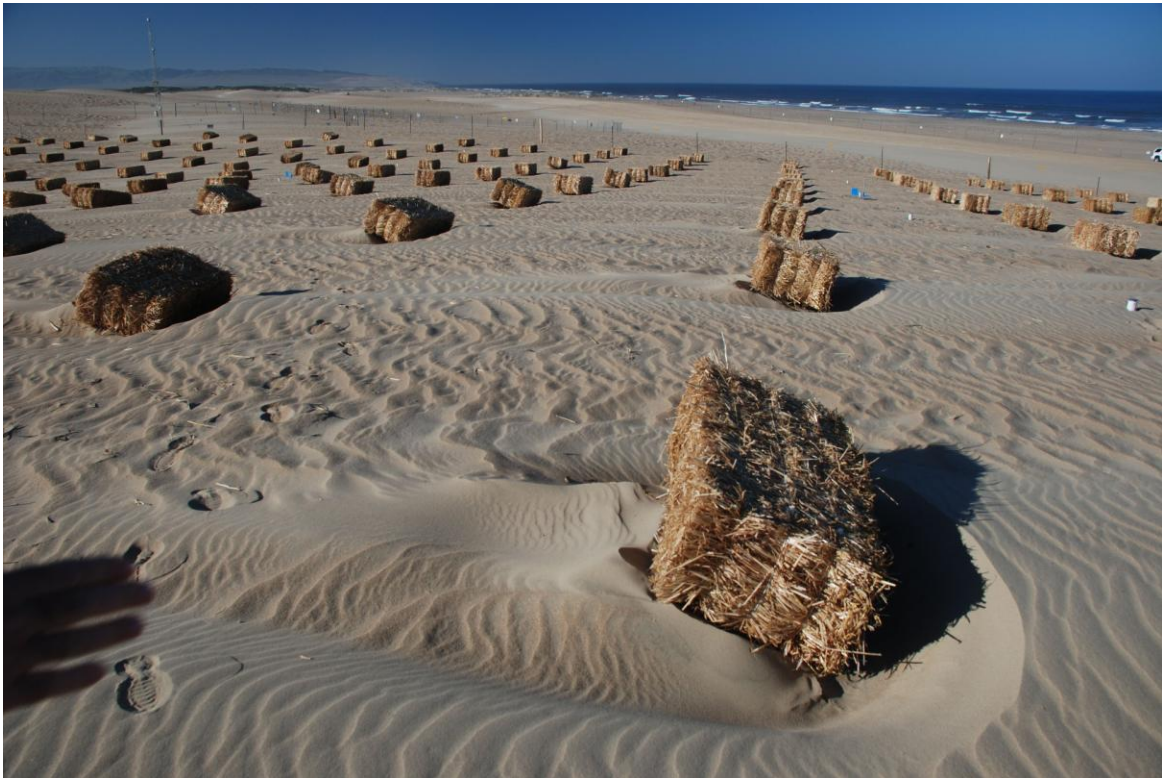
Figure 22. Scour and tilting of the straw bales following installation.
