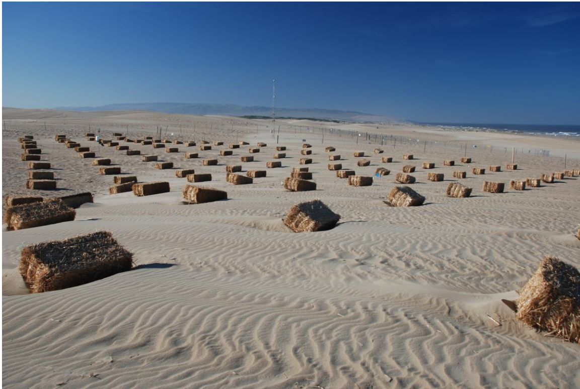
Figure 3. Straw Bale Roughness Demonstration Plot – view to southeast and S1 tower.
