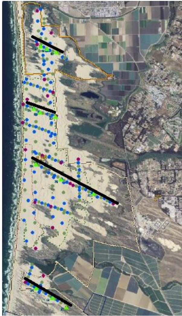
Figure 14. Four Transects Used for Measurements at the ODSVRA (Transects are shown with black lines, with Transect #1 at the top, progressing downward to Transect #4 at the bottom. Green triangles show each wind site. Transects 1&4 are located in non-riding areas; Transects 2 & 3 are located within the riding areas.)
