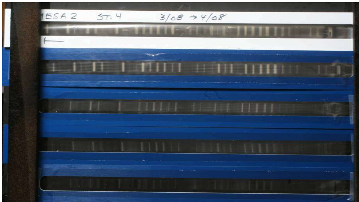
Figure C 58 - 8 DRUM strips for the coarsest 5 fractions (from top to bottom) for the March-April intensive period. The white lines are dust episodes
