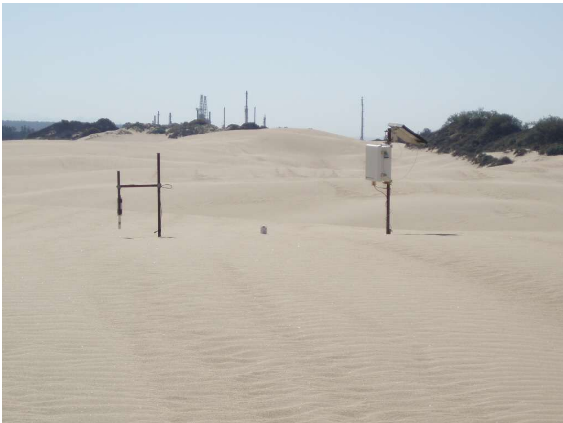
Figure 2.7 - Site C2 with Sensit, Cox Sandcatcher, and Datalogger
