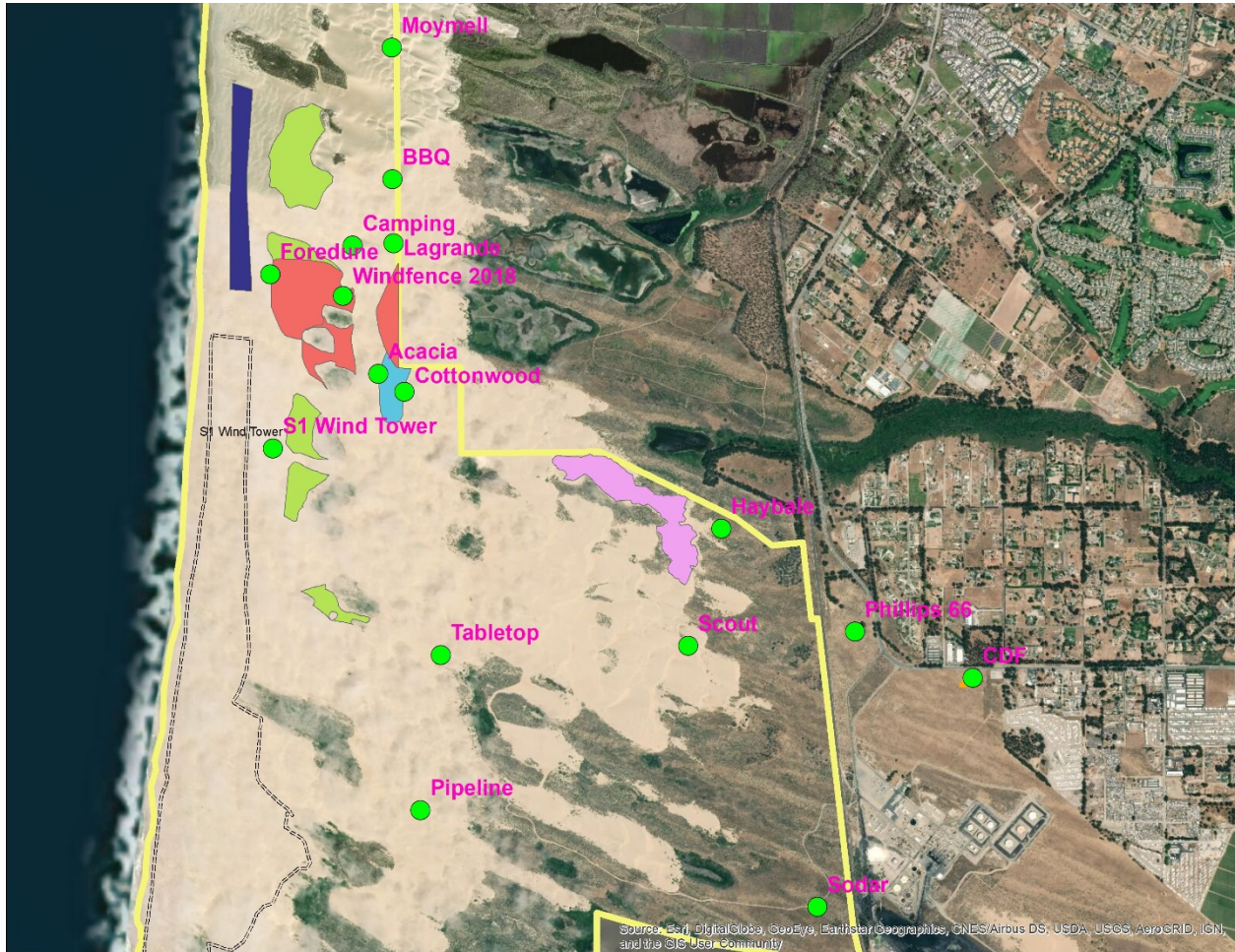
Figure 1. The locations of PM and met stations in 2019. The configuration was the same in 2018, with 2019 adding the stations: Moymell, Tabletop, Scout, Pipeline, and Sodar. The blue rectangle approximates the position of the foredune restoration area.
