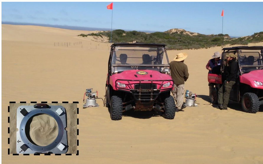
237 Figure 2. Collocation of two PI-SWERL units. Inset shows the test plate that the PI-SWERL was placed 238 upon.
