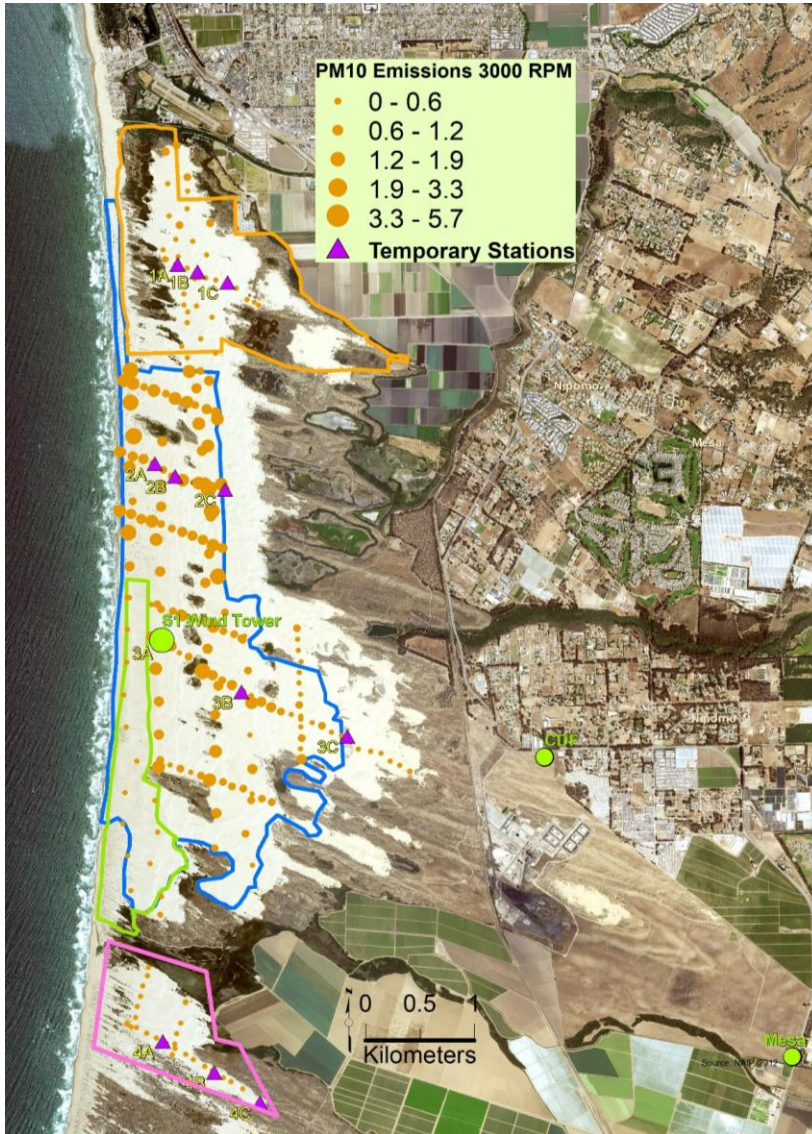
549 Figure 5. Spatial distribution of PI-SWERL measured PM 10 emissions (mg of PM 10 m -2 s -1 ) at 3000 RPM, 550 which is equivalent to u_* = 0.53 \text{ m s}^{-1} .
